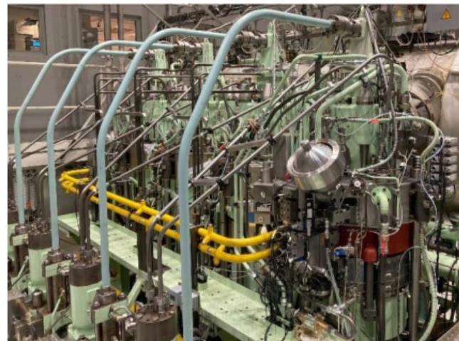
Figure 3. Photo of cylinder cover for ammonia tests mounted on the MAN B&W 4T50ME-X test engine in Copenhagen.
