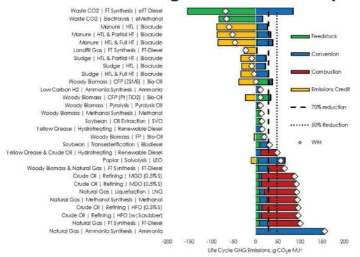
CFP: Catalytic Fast Pyrolysis; ZSM5: Zeolite Socony Mobil-5; TiO2: Titanium Dioxide; PF: Fast Pyrolysis; HTL: Hydrothermal Liquefaction; HT: Hydrotreating; LFG: Landfill Gas; SVO: Straight Vegetable Oil; LFO: Lignin Ethanol Oil; MGO: Marine Gas Oil; MDO: Marine Distillate Oil; HFO: Heavy Fuel Oil; LNG: Liquefied Natural Gas; FT: Fischer-Tropsch; S; Suffur; T&D: Transportation and Distribution; WHH: Well-to-Hull
