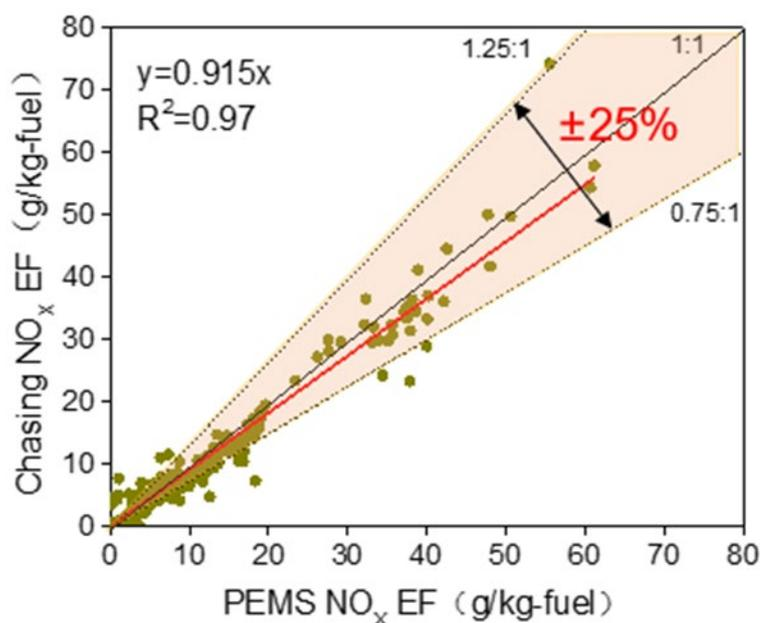
Fig. 1. The comparative tests of NO<sub>x</sub> emissions between RES Type 3 and PEMS (four vehicles, 360 chasing events in total).
