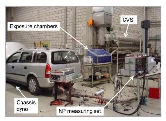
Fig. 1 Exposure Tests on a Diesel Passenger Car (CVS = constant volume sampling; NP = nanoparticle)
