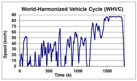
Fig. 1 World Harmonized Vehicle Cycle
