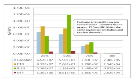
Fig. 2 Total Particulate Concentrations (#/cm<sup>3</sup>): 2.2-Liter DISI Engine
