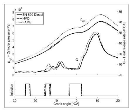
Fig. 1 Cylinder Pressure, Heat Release Rate, and Injection for HVO, FAME, and Reference Diesel (EN 590), n = 2,000min<sup>-1</sup>, p<sub>me</sub> = 9 bar
