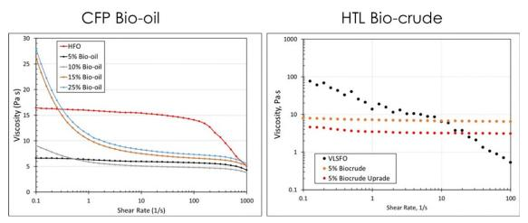
Figure 44 Viscosity versus shear rate for blends of bio-oil and bio-crude with VLSFO at 25°C.
