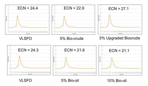
Figure 45 Estimated cetane number results for HTL bio-crude (top) and CFP bio-oil (bottom) as a function of blend level with VLSFO.
