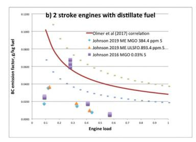
Figure 34 Comparison of Black Carbon data with emission factors from 2-stroke engines with distillate fuel
