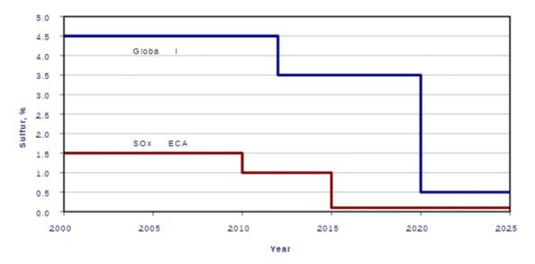
Figure 22: Sulfur limit in global waters and ECA zones. Illustration from Dieselnet.com
