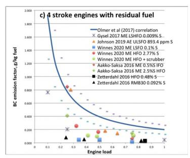
Figure 35 Comparison of Black Carbon data with emission factors from 4-stroke engines with residual fuel
