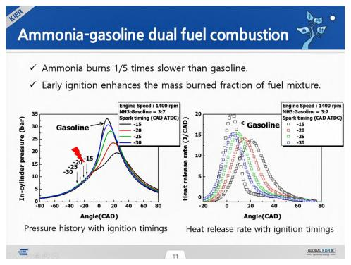
Figure 75 Slow burning is a principal feature of ammonia when used as a fuel.
