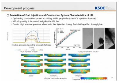
Figure 15 Injection and ignition processes with some advanced marine fuels
