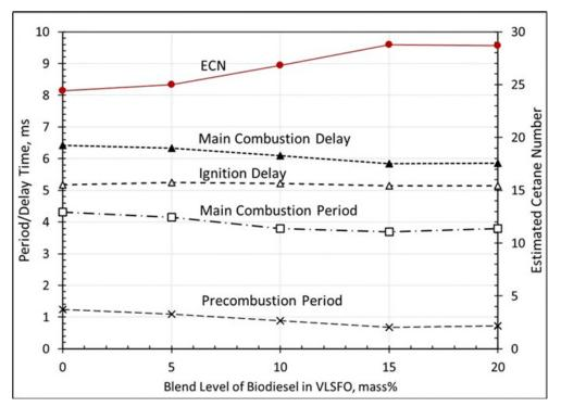
Figure 49 Estimated cetane number and combustion properties for biodiesel blends with VLSFO.
