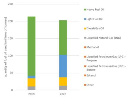
Figure 26: Fuel oil consumption reported for ships above 5000GT in 2019 and 2020. Figure from IMO document MEPC 77/6/1 - Report of fuel oil consumption data submitted to the IMO Ship Fuel Oil Consumption Database in GISIS (Reporting year: 2020)
