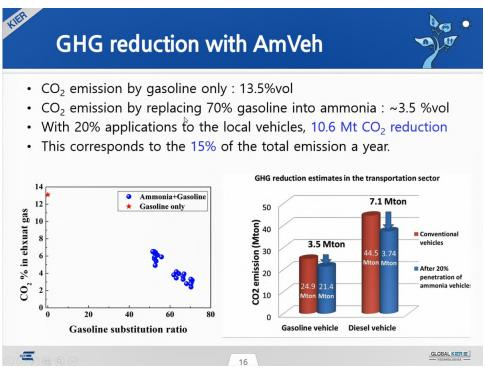
Figure 80 Engine-out  $CO_2$  can be reduced by roughly 70% with ammonia.
