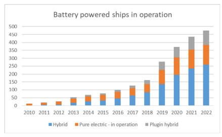
Figure 82: Development in battery powered ships. Source: DNV AFI
