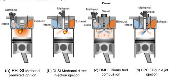
Figure 62 Methanol combustion concepts
