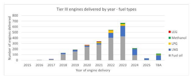
Figure 25: 2-stroke Tier III engine fuel design deliveries by year
