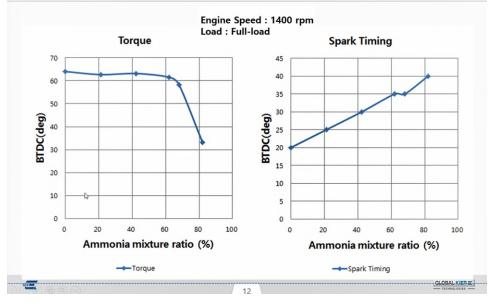
Figure 76 Mixtures above 60% ammonia reduce engine performance.
