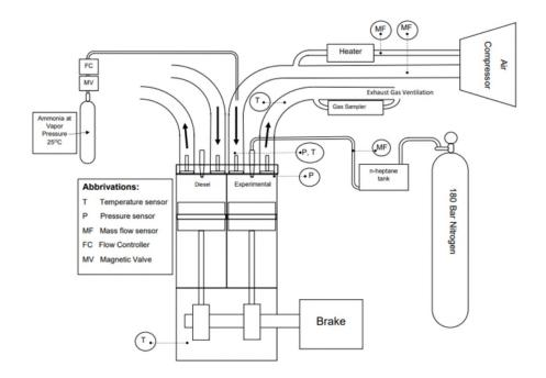
Figure 64 DTU Test engine set-up.
