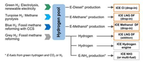
Figure 38 Hydrogen pathways for ICE include fuels compatible with common diesel and gas engines : hydrogenbased e-fuels as drop-in.
