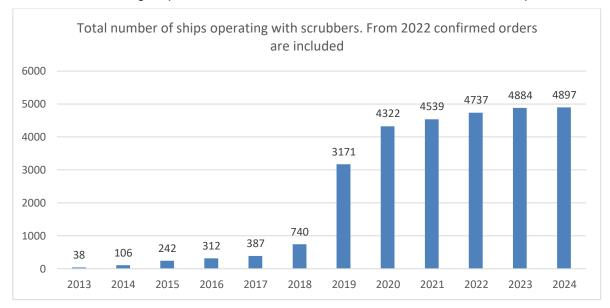
According to the DNV AFI, about 67 % of ships operating with scrubbers have been retrofitted to existing ships, while 33 % of the installations are made on new ships.
