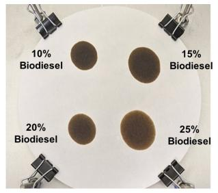
Figure 46 ASTM 4740 test results for biodiesel blends with VLSFO.
