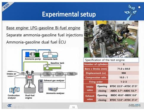
Figure 74 A dual fuel stoichiometric port injected ammonia-gasoline engine.
