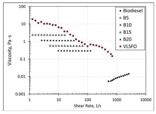
Figure 48 Dynamic viscosity of VLSFO with biodiesel additions up to 20%.
