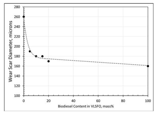
Figure 47 Wear scar diameter measurements for biodiesel blends with VLSFO. Results show a significant reduction in wear scar diameter (improved lubricity) with added biodiesel.
