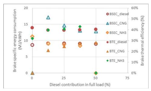
Figure 8 Brake specific energy consumptions and thermal efficiencies from ammonia-CNG-diesel triple fuel combustion at full load condition.
