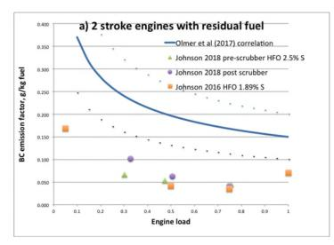
Figure 33 Comparison of Black Carbon data with emission factors from 2-stroke engines with residual fuel
