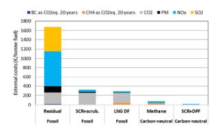
Figure 40 Examples of external costs of ship emissions with selected technologies.GWP20 values were used for methane and BC emissions.
