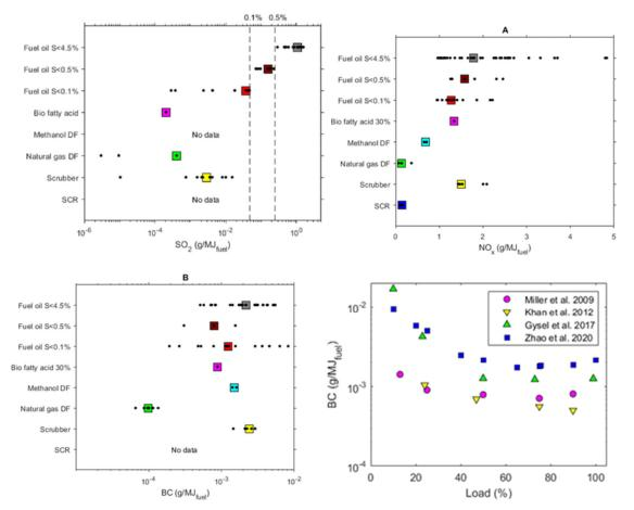
Figure 39 BC, NO<sub>X</sub> and SO<sub>2</sub> emissions per MJ fuel
