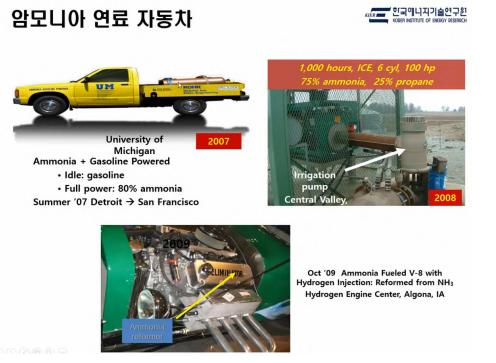
Figure 72 Ammonia can be used in dual-fuel applications with gasoline or propane, or directly in hydrogen engines by reforming of  $NH_3$  to  $H_2$ .
