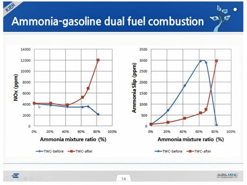
Figure 78 Mixtures above 60% ammonia lead to higher NOx and ammonia emissions.
