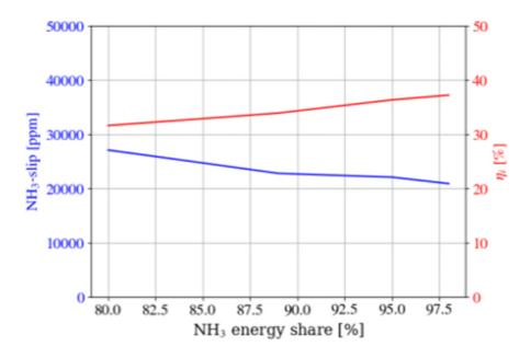
Figure 67 Ammonia-slip and indicated efficiency  $\eta_i$  vs. ammonia energy share with constant  $\lambda$  = 1.1.  $\eta_i$ =28,3% with pure diesel operation)
