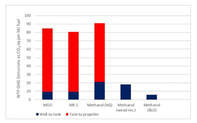
Figure 60 GHG emissions per MJ fuel for methanol from natural, wood residues, and black liquor gasification (BLG) as compared to marine gasoil and MK 1 diesel. (Ellis et al., 2018).
