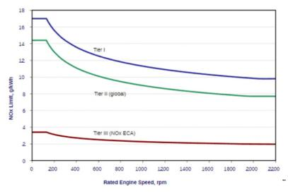
Figure 23: NOx emission limit for Tier I, II and III. Illustration from Dieselnet.com
