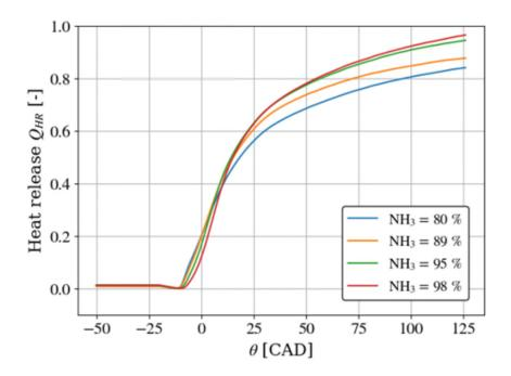
Figure 66 Integrated heat release curves with increasing ammonia energy and constant  $\lambda$  = 1.1, normalized by the total fuel energy and shifted to begin combustion from 0 heat released.
