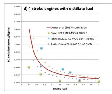
Figure 36 Comparison of Black Carbon data with emission factors from 4-stroke engines with distillate fuel
