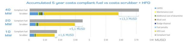
Figure 30: Accumulated costs calculated for different scrubber sizes assuming a 200 USD fuel price spread. Source: (DNV-GL , 2018)
