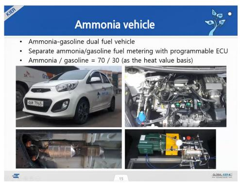
Figure 79 A working dual fuel ammonia-gasoline vehicle.
