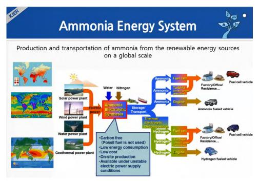
Figure 69 Ammonia can serve directly as a fuel or as a hydrogen carrier.
