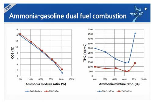
Figure 77 Mixtures above 60% ammonia lead to higher unburnt hydrocarbon emissions.
