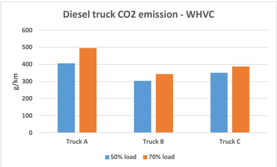
Figure 53: Diesel truck CO<sub>2</sub> emissions, hot WHVC.
