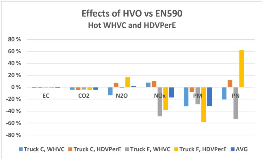
Figure 79: Effects of HVO on diesel truck performance (reference EN590).
