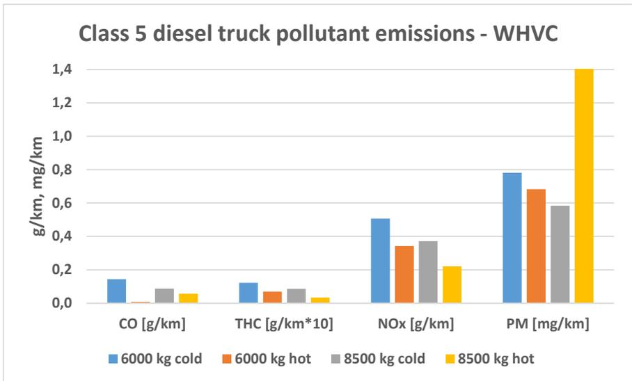
**Figure 42: Class 5 diesel truck pollutant emissions, WHVC in g/km, ULSD fuel. PM for 8500 kg hot 2.9 mg/km.**
