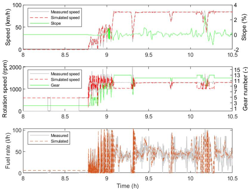
**Figure 31: Measured and simulated values for the simulation model validation: vehicle speed, engine speed and fuel rate.**
