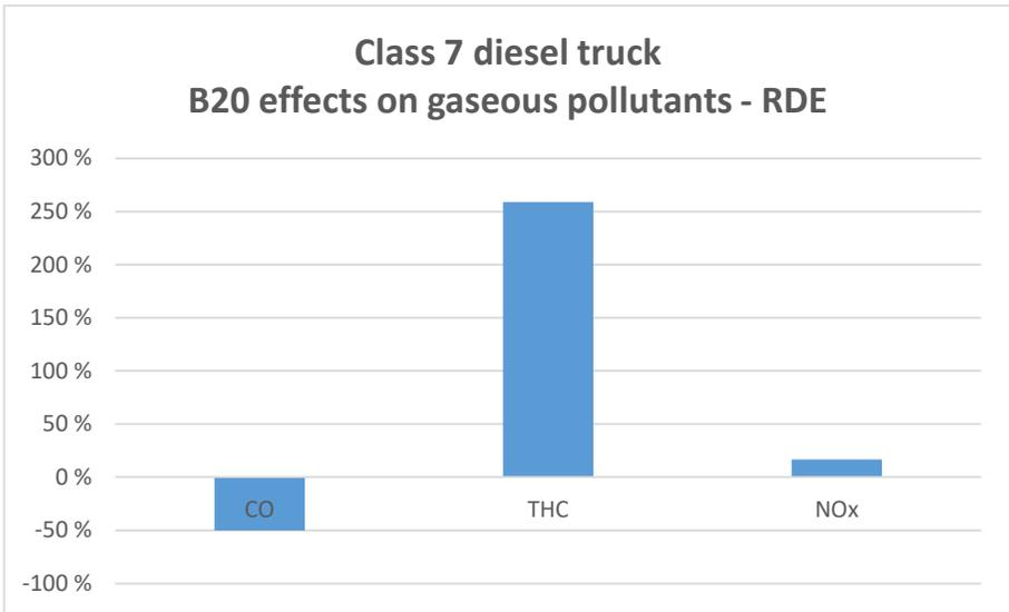
**Figure 50: Effect of B20 on gaseous pollutant emissions, RDE, high load (reference ULSD).**
