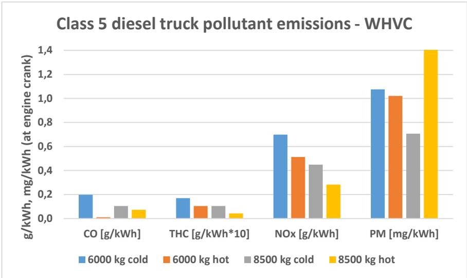
Figure 43: Class 5 diesel truck pollutant emissions, WHVC in g/kWh, ULSD fuel. PM for 8500 kg hot 3.7 mg/kWh.
