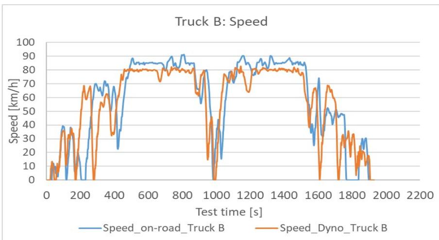
**Figure 80: Speed profile comparison between measurements on-road and chassis dynamometer, truck B.**
