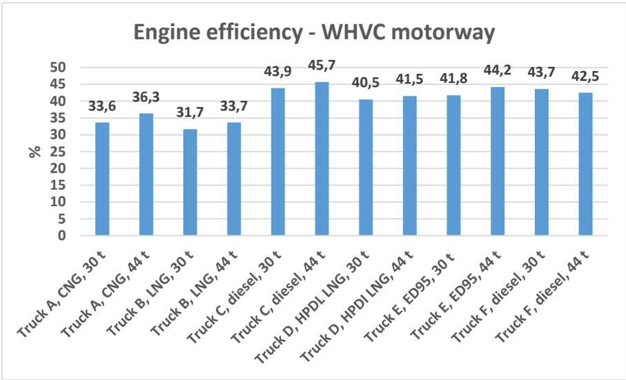
Figure 62: Engine efficiency for the WHVC motorway part.
