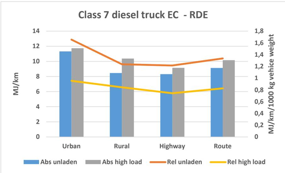
**Figure 39: Class 7 diesel truck energy consumption (RDE, unladen and high load).**
