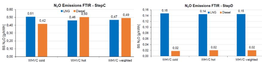
Figure 100: N<sub>2</sub>O emissions, Step C and D vehicles.
