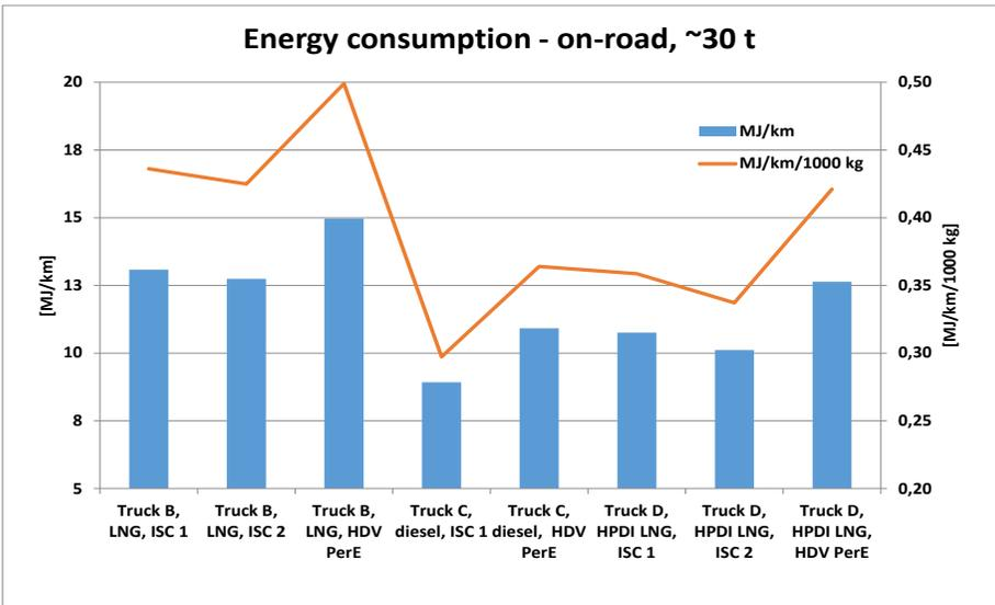
Figure 61: Energy consumption (on-road measurements, ~30 t).
