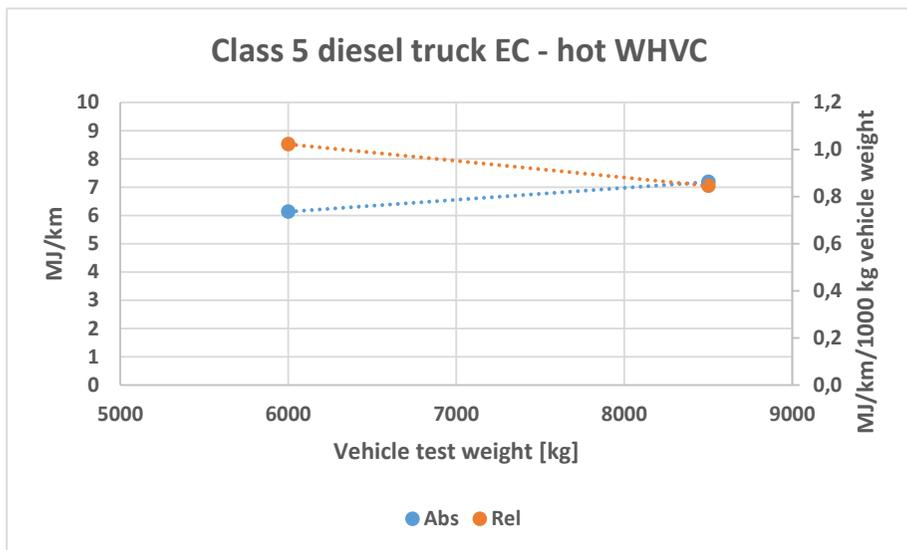
Figure 37: Class 5 diesel truck energy consumption (hot WHVC, medium and high load).
