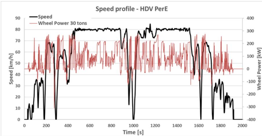
**Figure 26: VTT's HDVPerE test cycle.**
