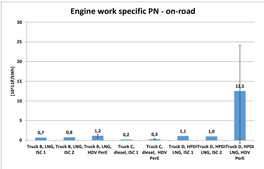
Figure 77: PN emissions (on-road measurements, g/kWh relative to engine work).
