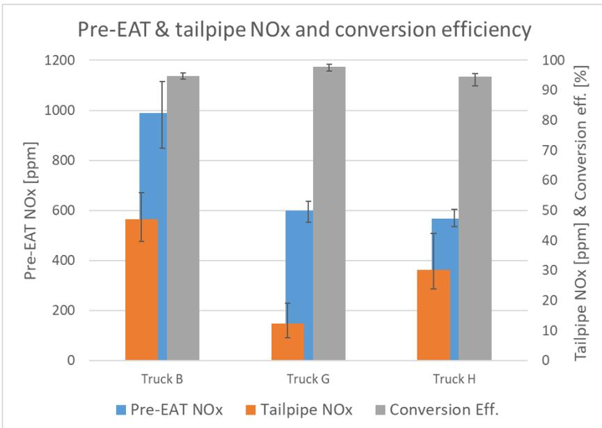
**Figure 82: Average pre- and post-EAT tailpipe NO<sub>x</sub> concentration and conversion efficiency during the monitoring period.**
