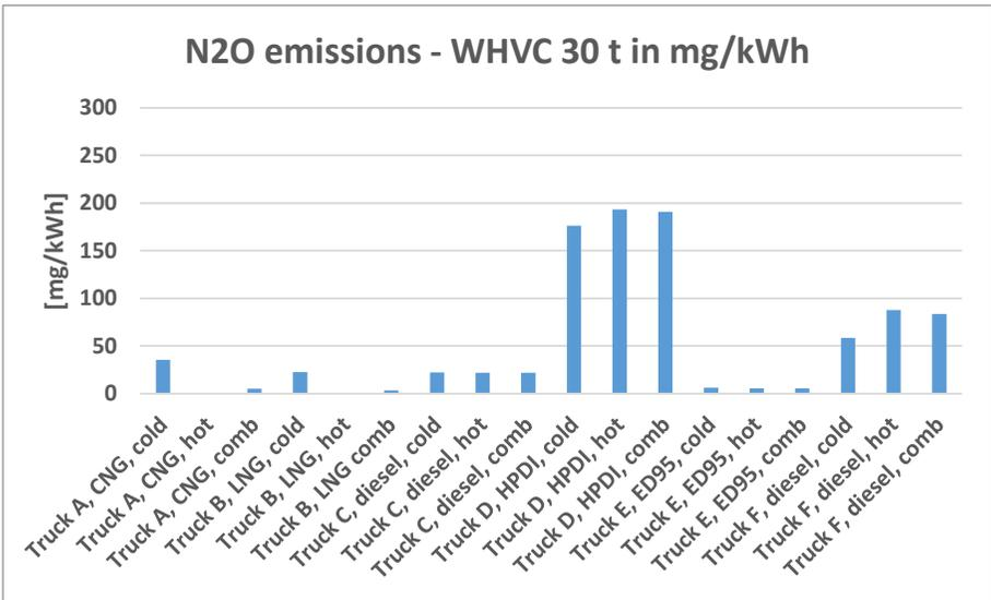
**Figure 67: N<sub>2</sub>O emissions (cold and hot WHVC, 30 t). Values relate to work at the driving wheels.**
