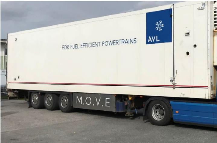
**Figure 29: Special semi-trailer used by AVL MTC for on-road PEMS measurements.**
