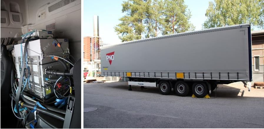
**Figure 27: PEMS device installation and semi-trailer used for the on-road measurements.**
