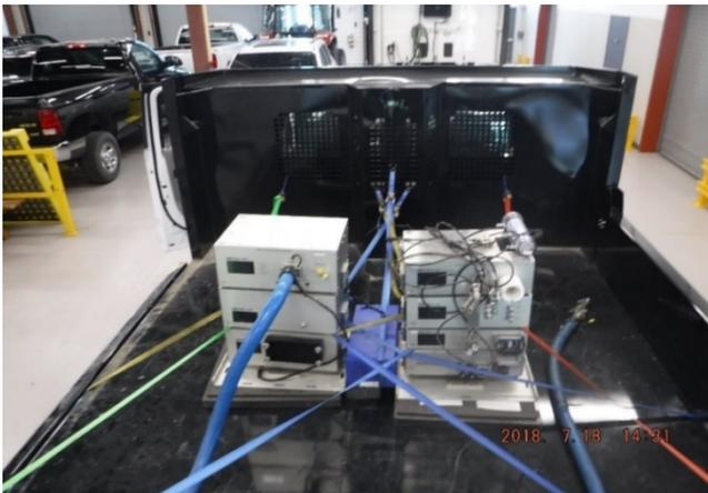
**Figure 22: PEMS setup in the open cab of the Class 5 test vehicle for on-road testing.**
