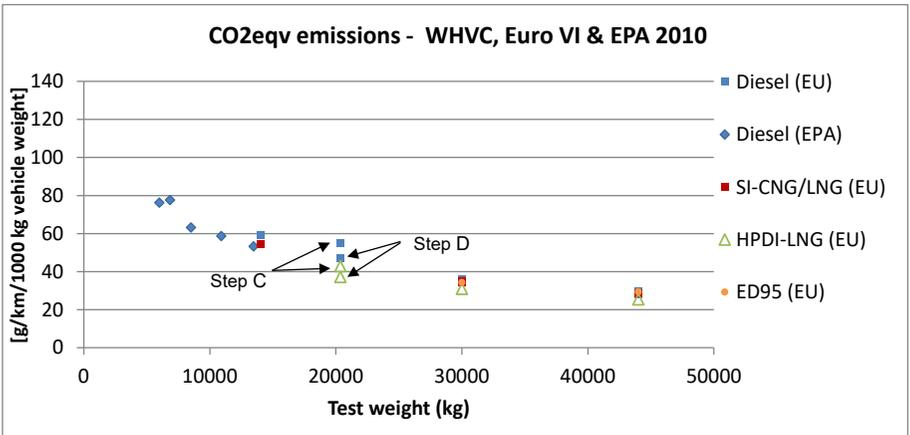
Figure 110: Ton-kilometer specific CO<sub>2</sub> equivalent emissions of Euro VI and EPA 2010 trucks.
