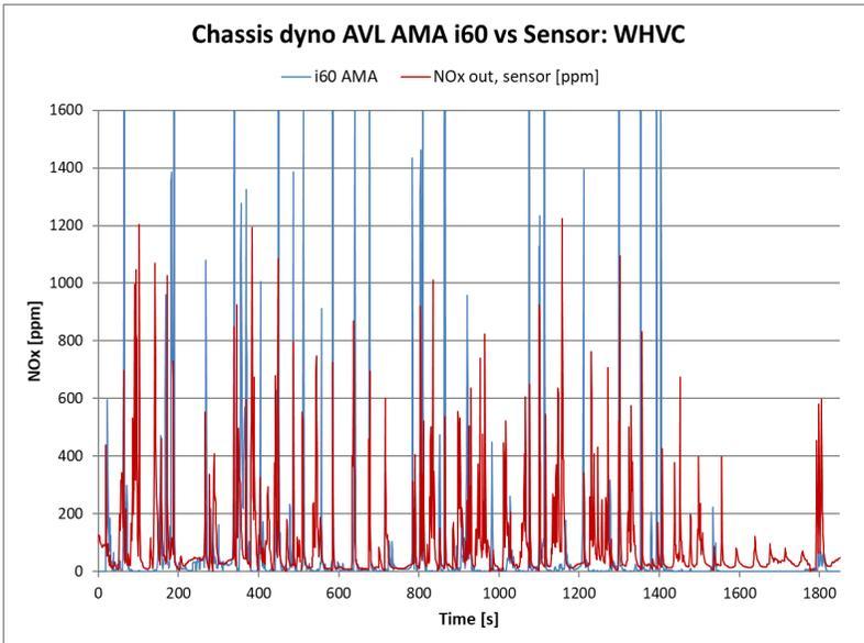
**Figure 85: Comparison of PROCARE Drive and AVL AMA i60 devices for NO<sub>x</sub> concentrations. Hot WHVC chassis dynamometer test.**
