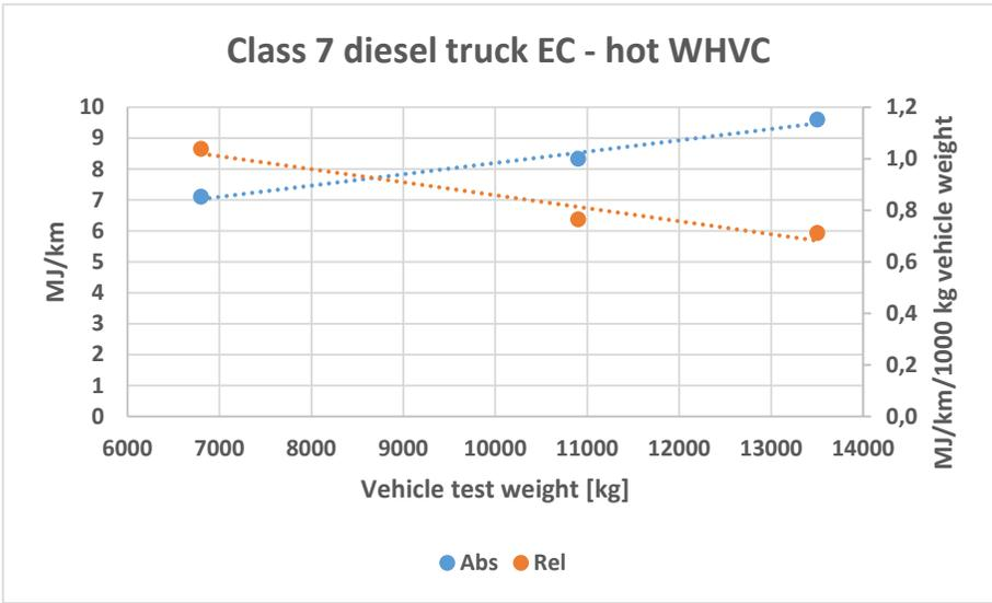
**Figure 38: Class 7 diesel truck energy consumption (hot WHVC, unladen, medium and high load).**
