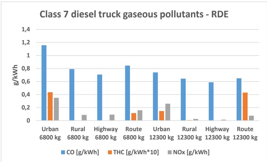
**Figure 49: Class 7 diesel truck gaseous pollutant emissions, RDE in g/kWh, unladen and high load.**
