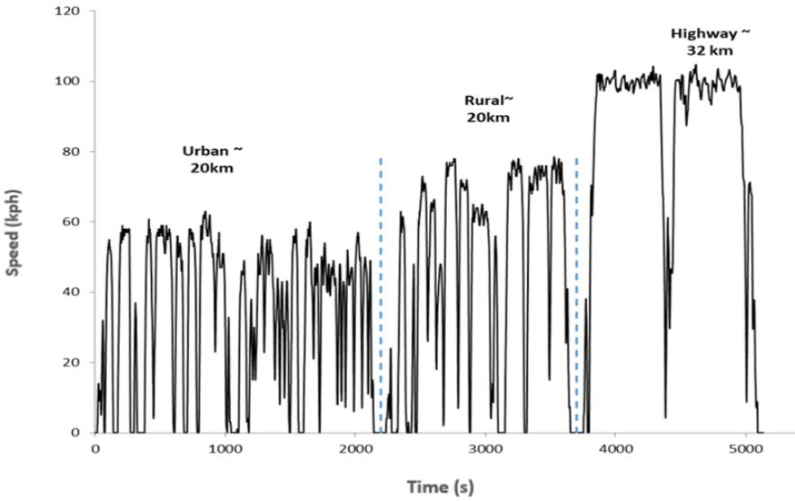
**Figure 23: Sample speed versus time trace of the RDE route.**
