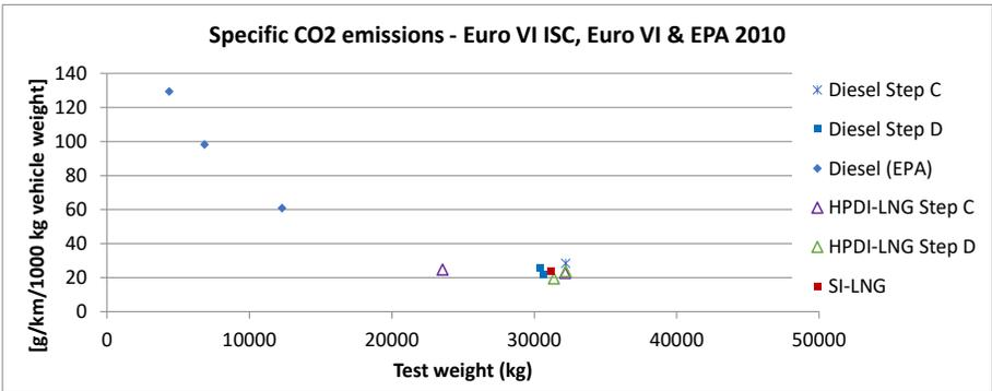
Figure 121: On-road ton-kilometer specific CO<sub>2</sub> emissions (Euro VI ISC route).
