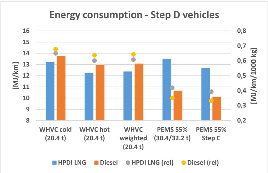
Figure 96: Energy consumption, Step D vehicles (Step C as a reference).
