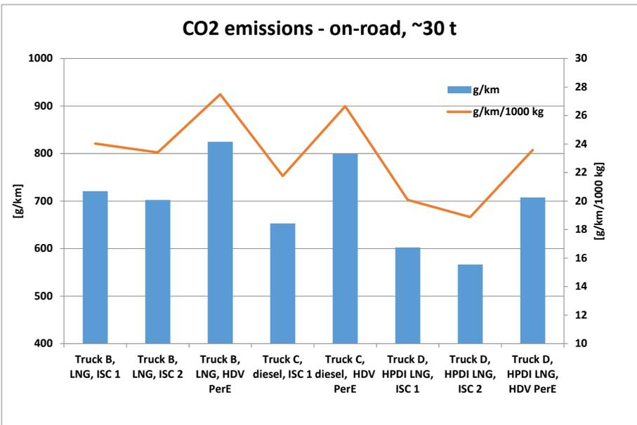
Figure 69: CO<sub>2</sub> emissions (on-road measurements, ~30 t).
