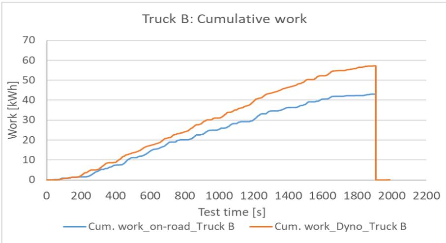
**Figure 81: Comparison of cumulative work on engine between measurements on-road and chassis dynamometer, truck B.**
