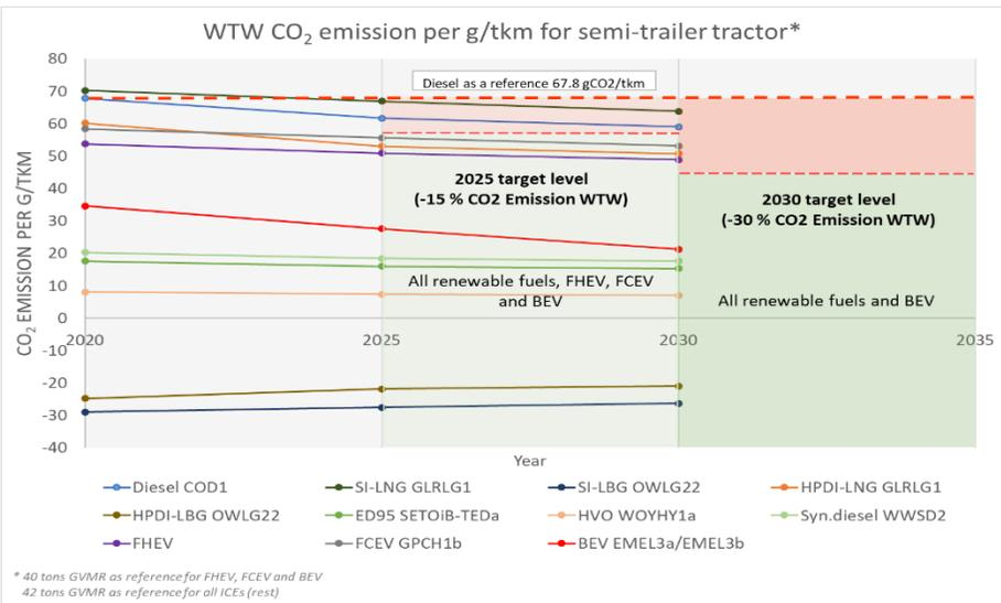
**Figure 132: CO<sub>2</sub> emissions in WTW basis per ton-kilometer for different powertrain and fuel options.**
