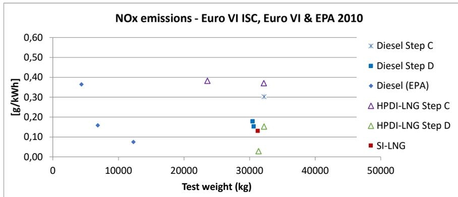
Figure 123: On-road engine work specific NO<sub>x</sub> emissions (Euro VI ISC route).
