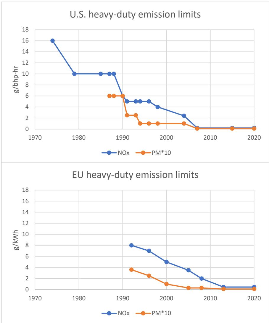
**Figure 8: The development of US and European NO<sub>x</sub> and PM values. Data from (DieselNet, 2020).**
