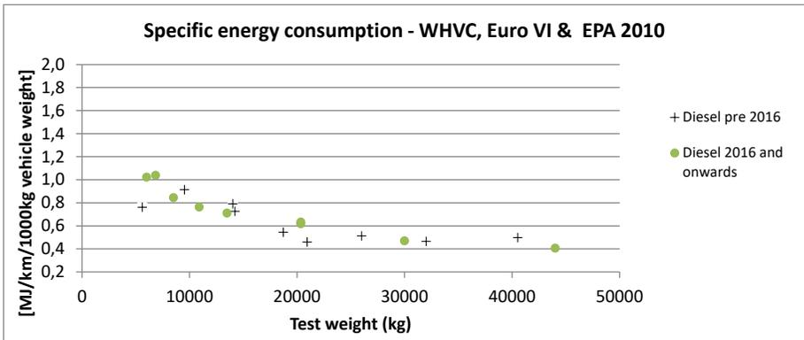
**Figure 119: Ton-kilometer specific energy consumption of pre 2016 and newer diesel trucks (Euro VI and EPA 2010 trucks).**
