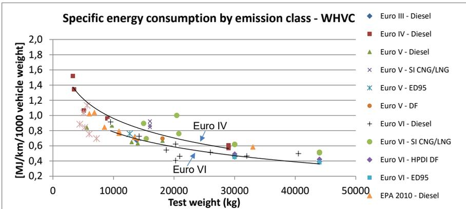
Figure 118: Ton-kilometer specific energy consumption of Euro III -VI, EPA 2010 and Chile 2015 trucks. Trendlines for Euro IV and Euro VI diesel vehicles.
