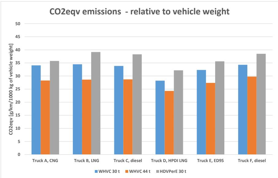
Figure 68: CO<sub>2eqv</sub> emissions relative to vehicle weight.
