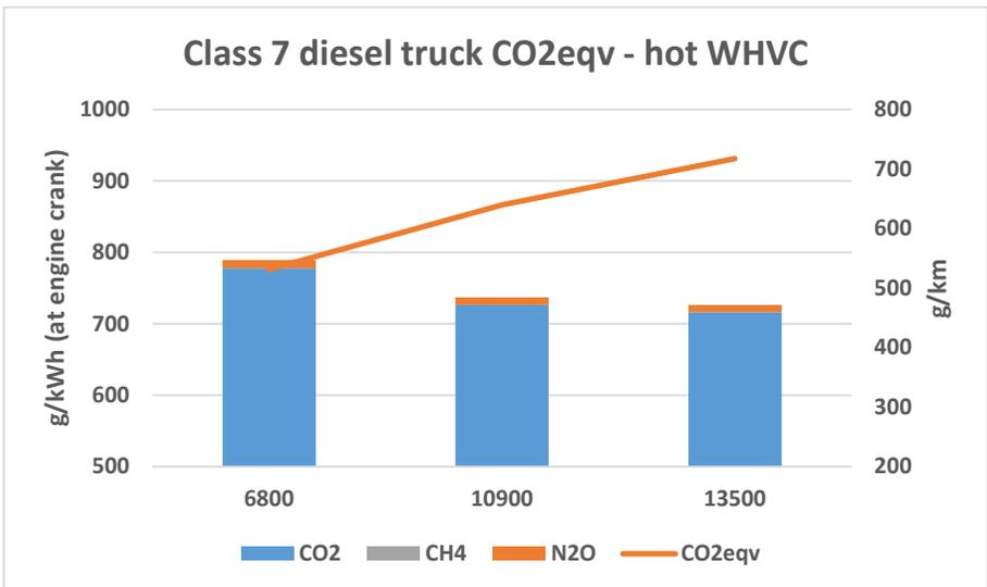
**Figure 41: Class 7 diesel truck CO<sub>2</sub>eqv emissions (hot WHVC, unladen, medium and high load).**
