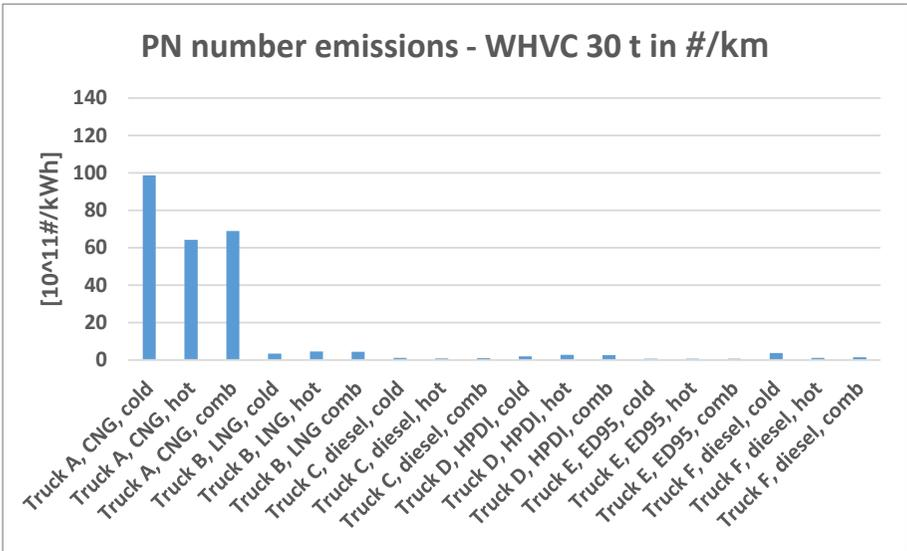
**Figure 74: PN emissions (cold and hot WHVC, 30 t). Values relate to work at the driving wheels.**
