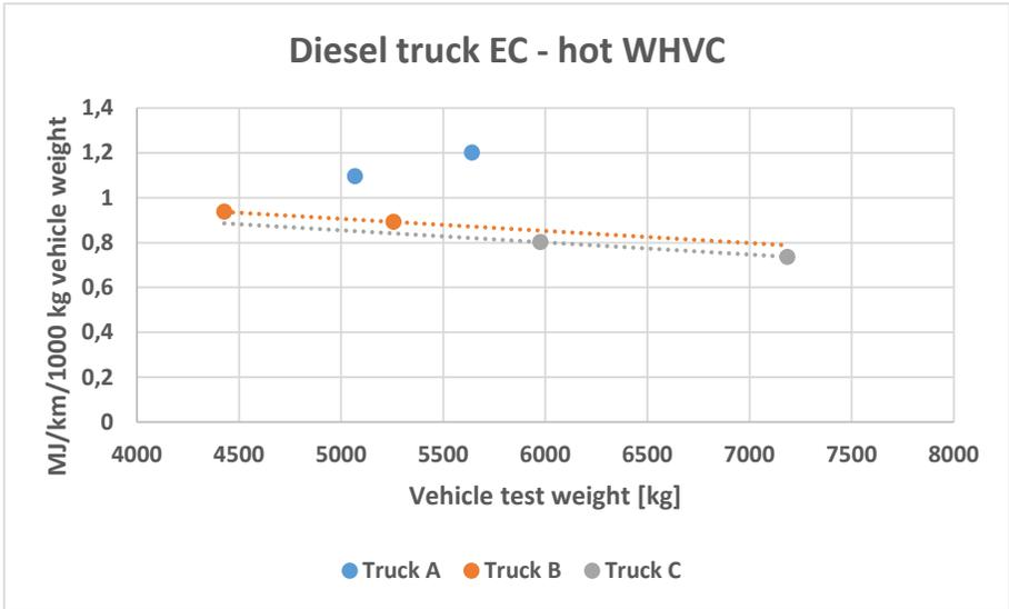
Figure 52: Diesel truck energy consumption relative to weight, hot WHVC.
