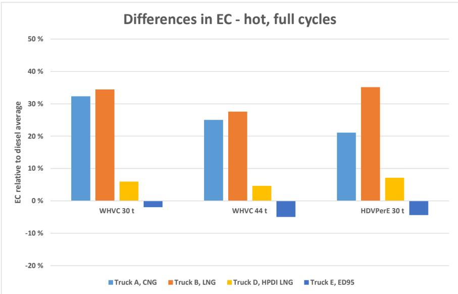
Figure 58: Energy consumption (hot testing, full cycles) relative to diesel average.
