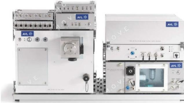
**Figure 28: AVL M.O.V.E PEMS system.**
