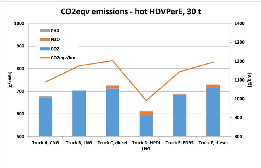
Figure 65: CO<sub>2</sub>eqv emissions (hot HDVPerE, 30 t). Values in g/kWh relate to work at the driving wheels.
