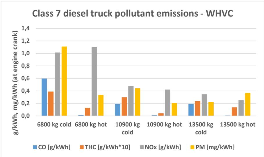
**Figure 45: Class 7 diesel truck pollutant emissions, WHVC in g/kWh, ULSD fuel.**
