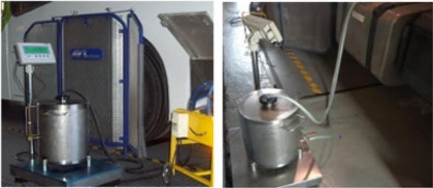
**Figure 25: Equipment for measuring fuel consumption gravimetrically.**
