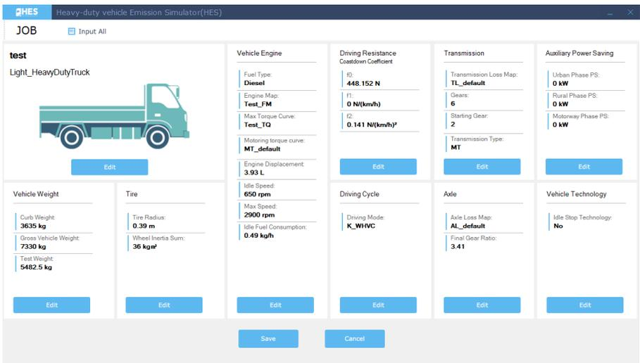
Figure 34: Example of HES user interface for adding the corresponding vehicle data.
