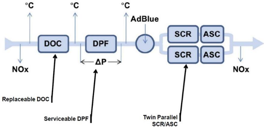
Figure 17: Schematics of the emission control system of a Euro VI diesel engine (Mackaldener, 2014). (DOC= diesel oxidation catalyst, DPF= diesel particulate filter, ASC= ammonia slip catalyst).
