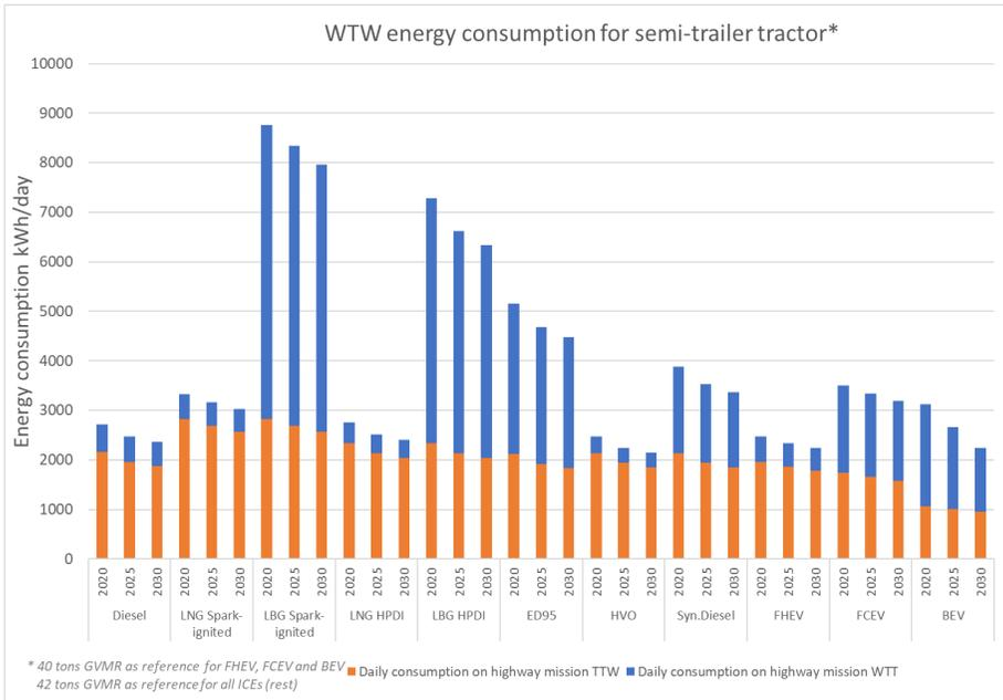
**Figure 133: Energy consumption in WTW (WTT+TTW) basis for different powertrain options.**
