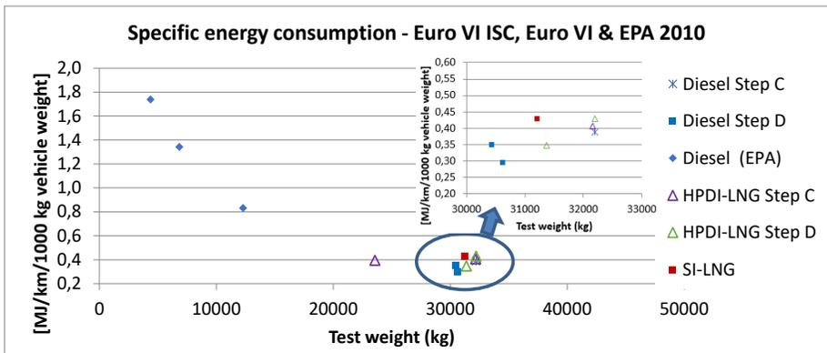
Figure 120: On-road ton-kilometer specific energy consumption (Euro VI ISC route).
