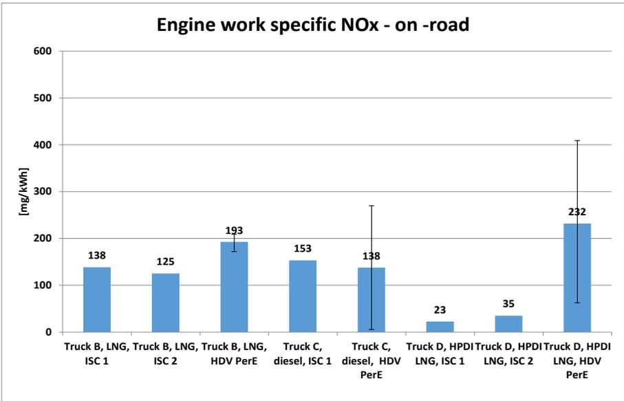
Figure 76: NO<sub>x</sub> emissions (on-road measurements, g/kWh relative to engine work).
