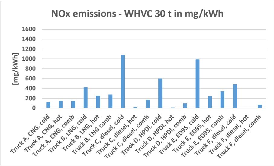
**Figure 70: NO<sub>x</sub> emissions (cold and hot WHVC, 30 t). Values relate to work at the driving wheels.**
