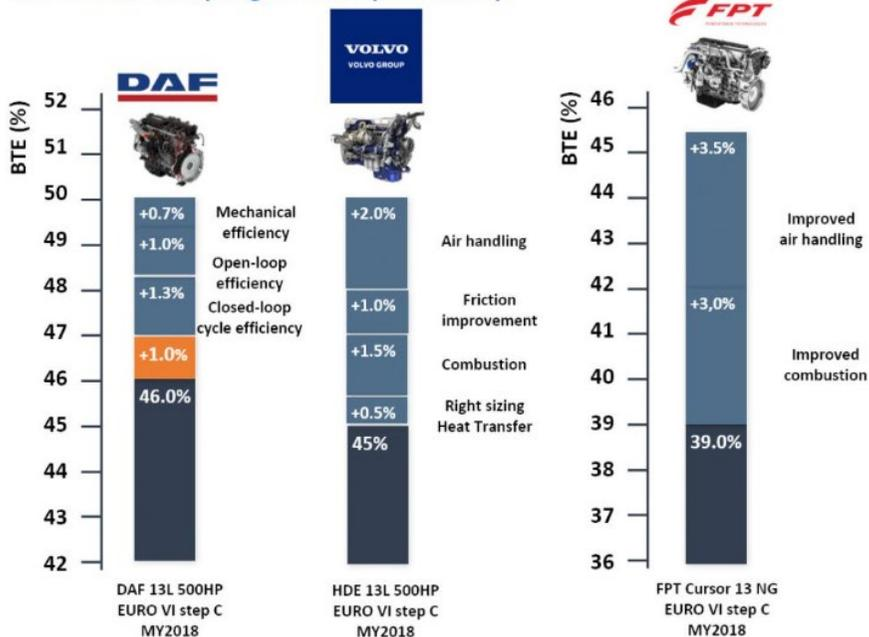
Figure 19: LONGRUN roadmap for engine efficiency (LONGRUN, 2020).
