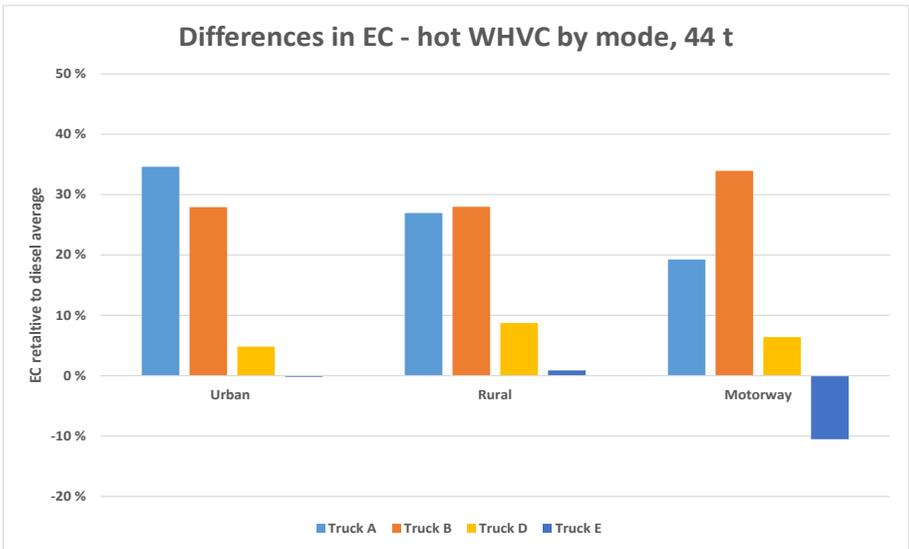
**Figure 60: Energy consumption (hot testing, WHVC 44 t by mode) relative to diesel average.**
