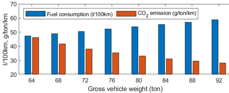
**Figure 124: Fuel consumption and specific CO<sub>2</sub> emission per ton-km as a function of gross vehicle weight.**
