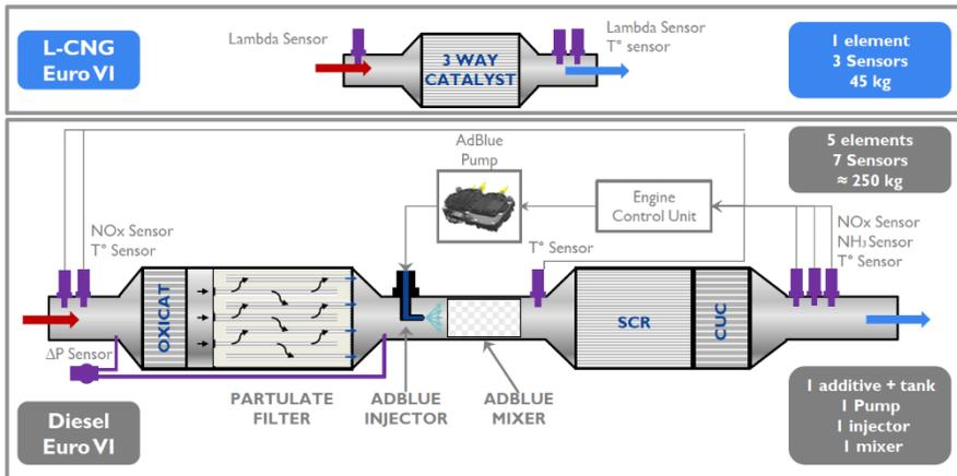
Figure 18: A comparison between Euro VI exhaust after-treatment systems for methane and diesel (Chandon, 2015).
