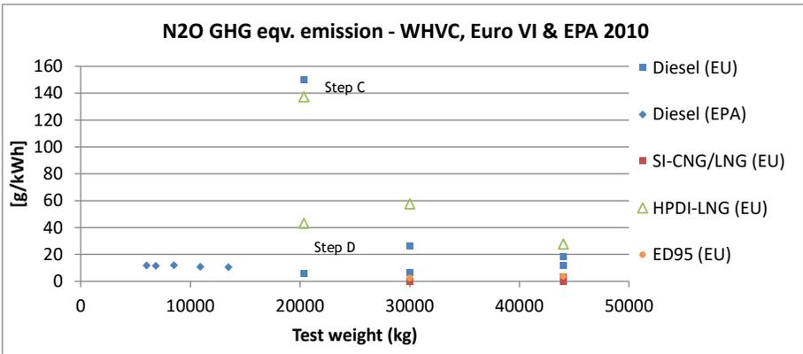
Figure 113: N<sub>2</sub>O (in CO<sub>2</sub>eqv) emissions of Euro VI and EPA 2010 trucks.
