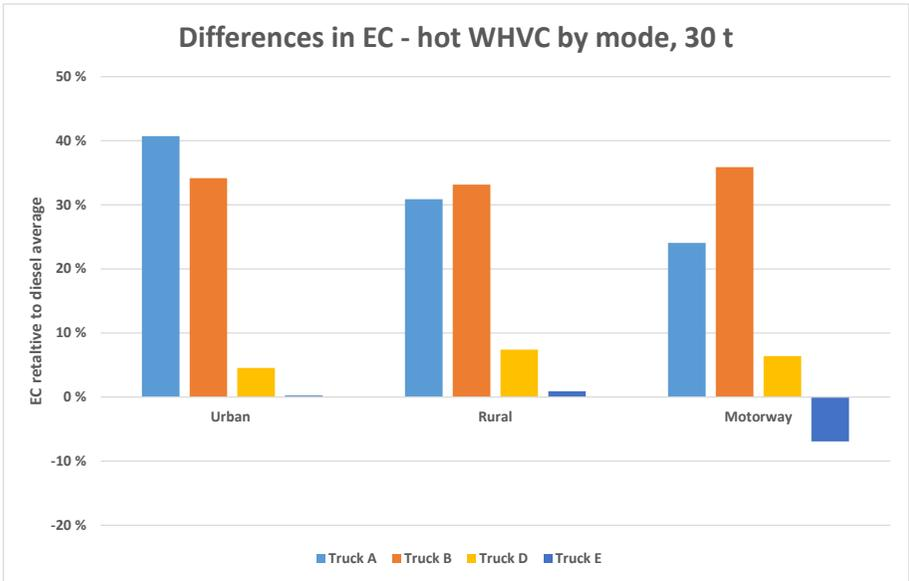
**Figure 59: Energy consumption (hot testing, WHVC 30 t by mode) relative to diesel average.**
