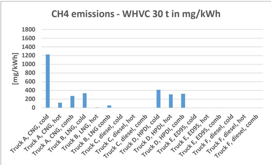
**Figure 66: CH<sub>4</sub> emissions (cold and hot WHVC, 30 t). Values relate to work at the driving wheels.**
