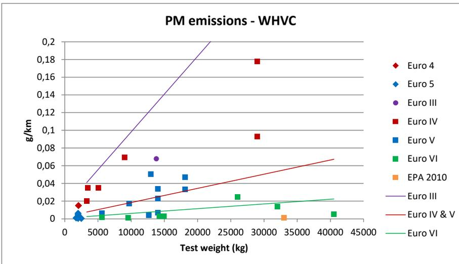
Figure 10: PM emission by emission class by emission class (IEA AMF, 2016a).
