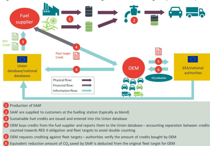
**Figure 134: Schematics of a CO<sub>2</sub> crediting system for renewable fuels.**
