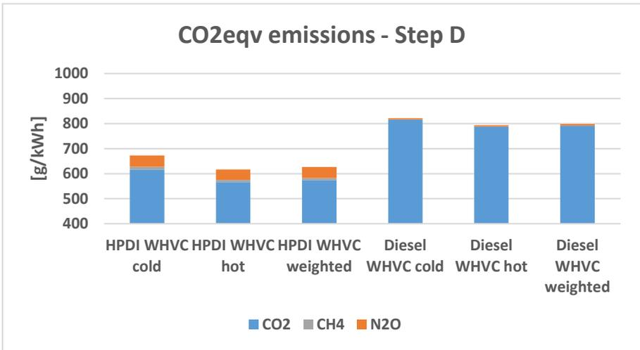
**Figure 102: CO<sub>2</sub>eqv emissions, Step D vehicles (values relative to engine work).**
