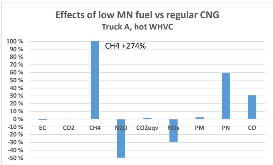
**Figure 78: Effects of low methane number gas on performance (reference pump quality CNG).**
