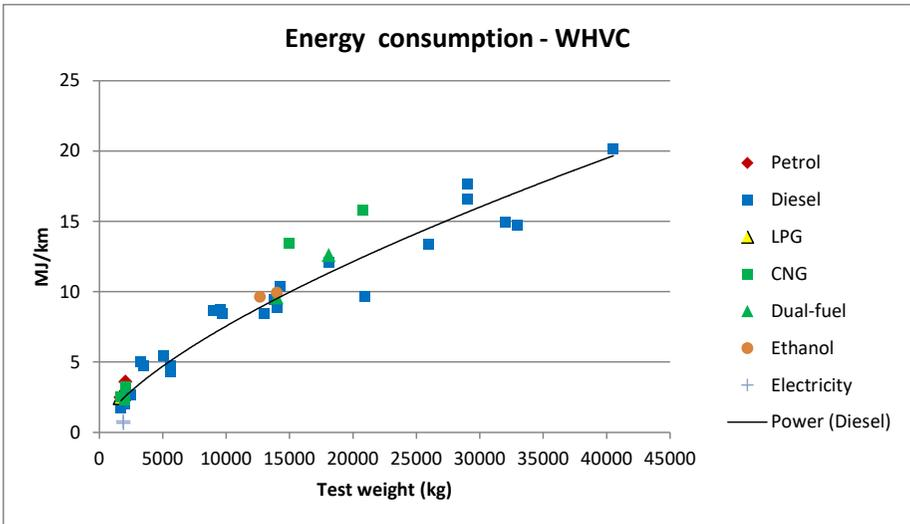
Figure 14: Energy consumption as a function of vehicle weight (IEA AMF, 2016a).
