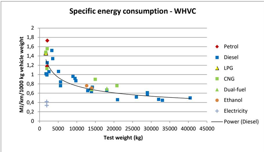
Figure 4: Specific energy consumption expressed in MJ per km per 1000 kg of vehicle weight (IEA AMF, 2016a).
