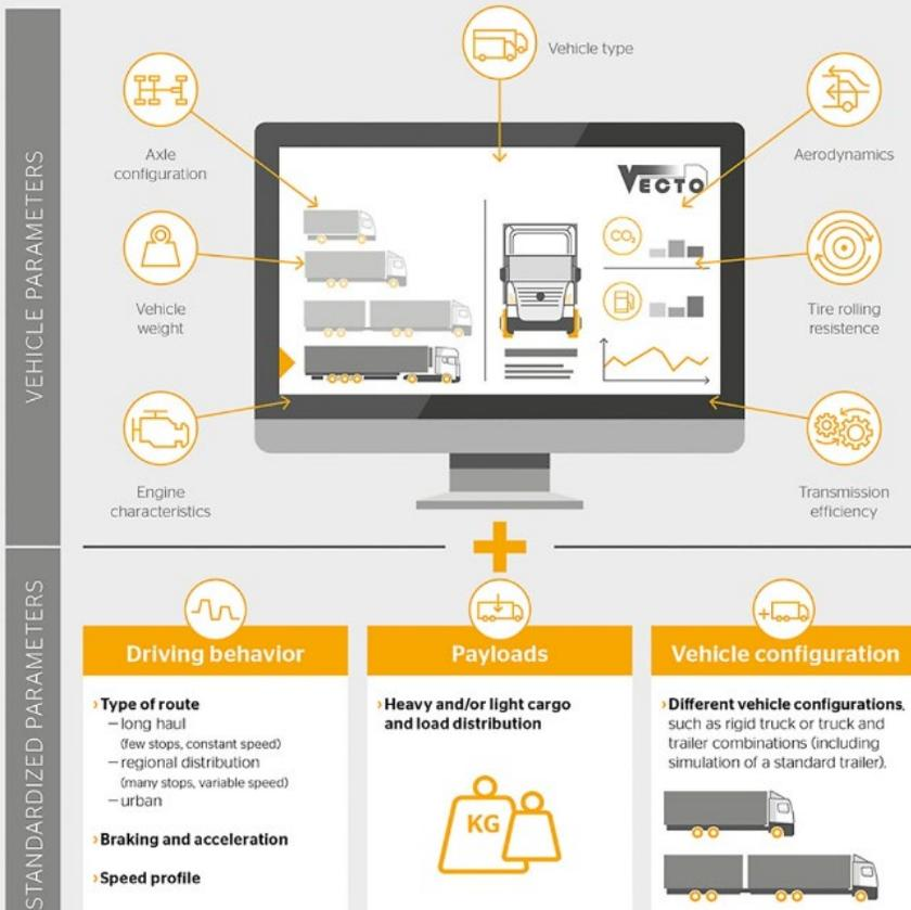
**Figure 6: Schematics of the European VECTO simulation system (European Union, 2019b).**
