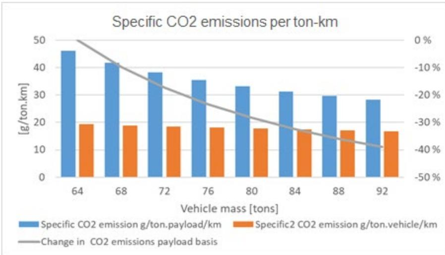
Figure 125: Ton-km specific CO<sub>2</sub> emissions in relation to vehicle mass and payload.
