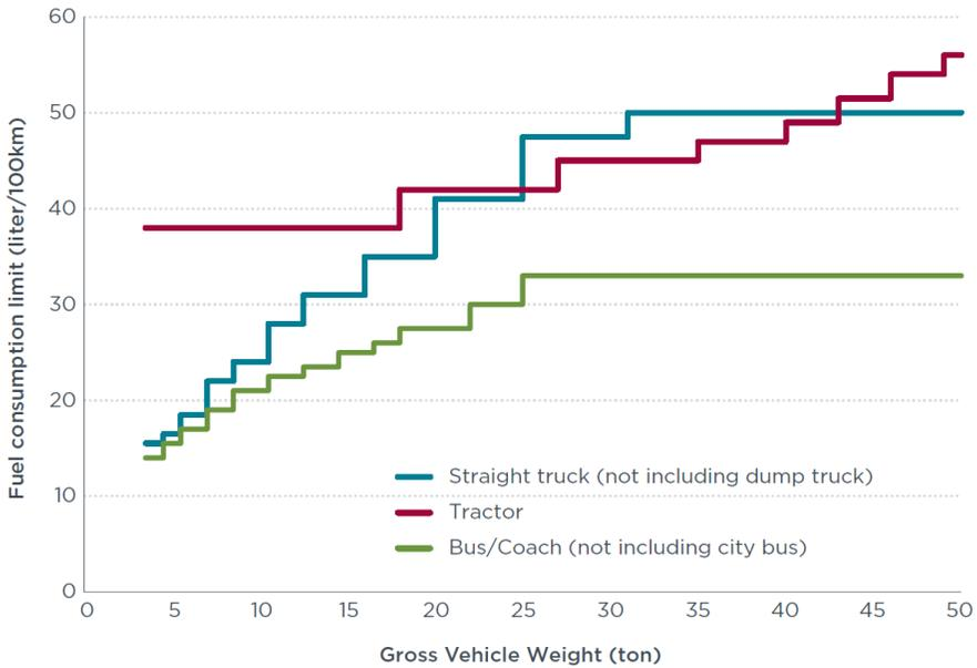
**Figure 7: Chinese 2012 - 2015 fuel consumption limits for heavy-duty vehicles (ICCT, 2013).**
