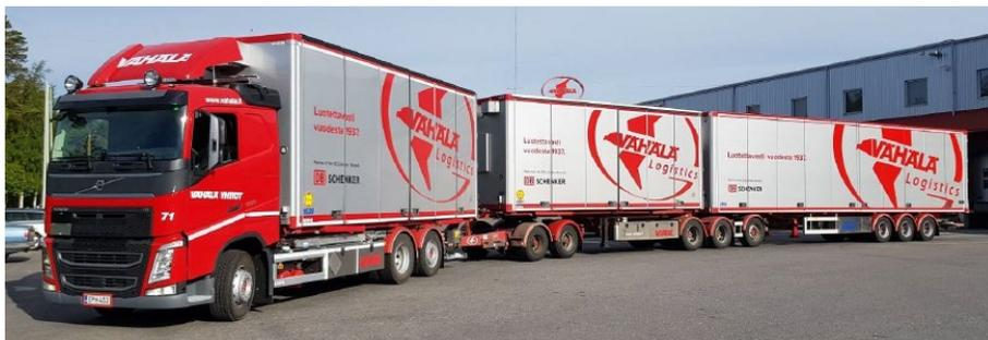
Figure 5: A 34.5 m long HCT vehicle combination (Lahti, 2019).
