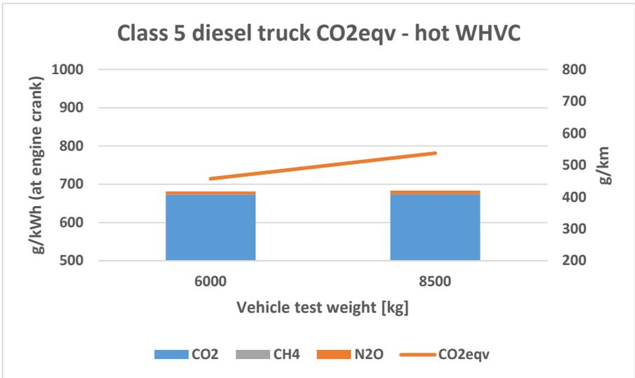
**Figure 40: Class 5 diesel truck CO<sub>2</sub>eqv emissions (hot WHVC, medium and high load).**
