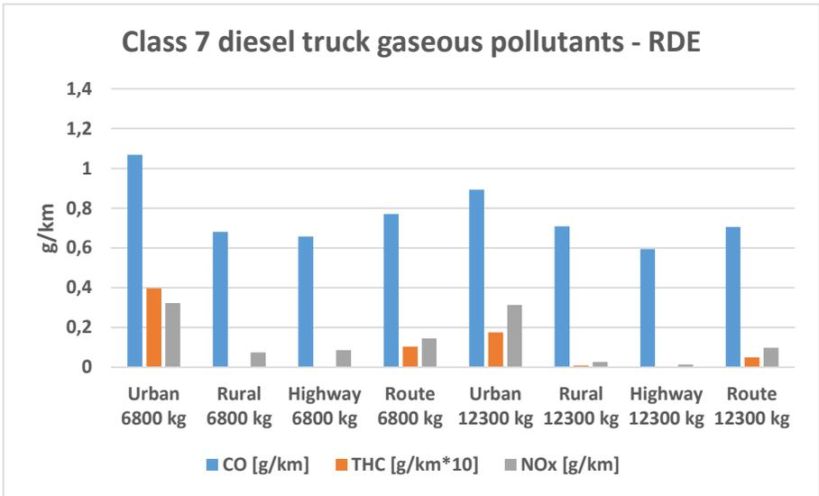
**Figure 48: Class 7 diesel truck gaseous pollutant emissions, RDE in g/km, unladen and high load.**
