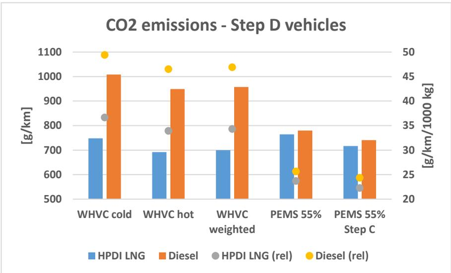
Figure 98: CO<sub>2</sub> emissions, Step D vehicles (Step C as a reference).
