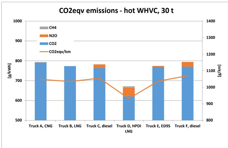
**Figure 63: CO<sub>2eqv</sub> emissions (hot WHVC, 30 t). Values in g/kWh relate to work at the driving wheels.**
