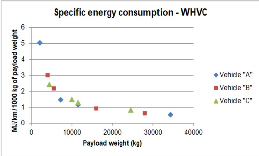
**Figure 36: The effect of load on specific energy consumption (MJ/1000 kg of payload) for heavy-duty trailer combinations. Source “COMVEC”.**
