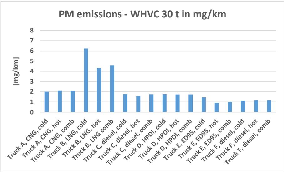
**Figure 72: PM emissions (cold and hot WHVC, 30 t). Values relate to work at the driving wheels.**
