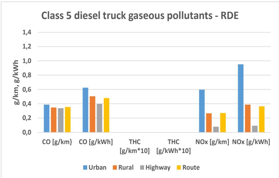
**Figure 47: Class 5 diesel truck pollutant emissions, RDE, unladen vehicle.**
