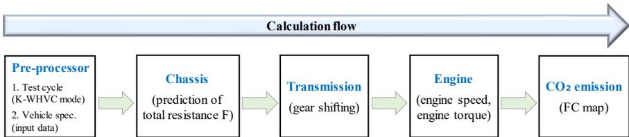
Figure 33: Calculation flow of HES model.
