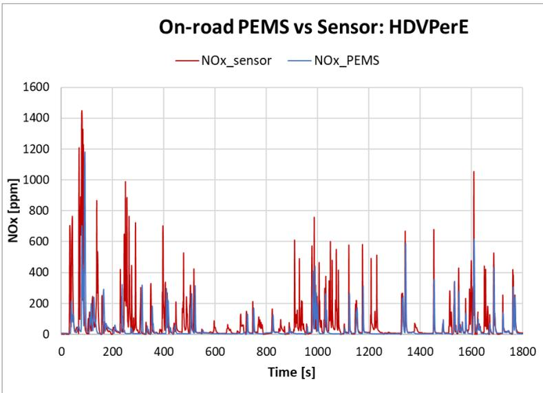
**Figure 84: Comparison of PROCARE Drive and PEMS devices for NO<sub>x</sub> concentrations. On-road test following the HDVPerE cycle.**
