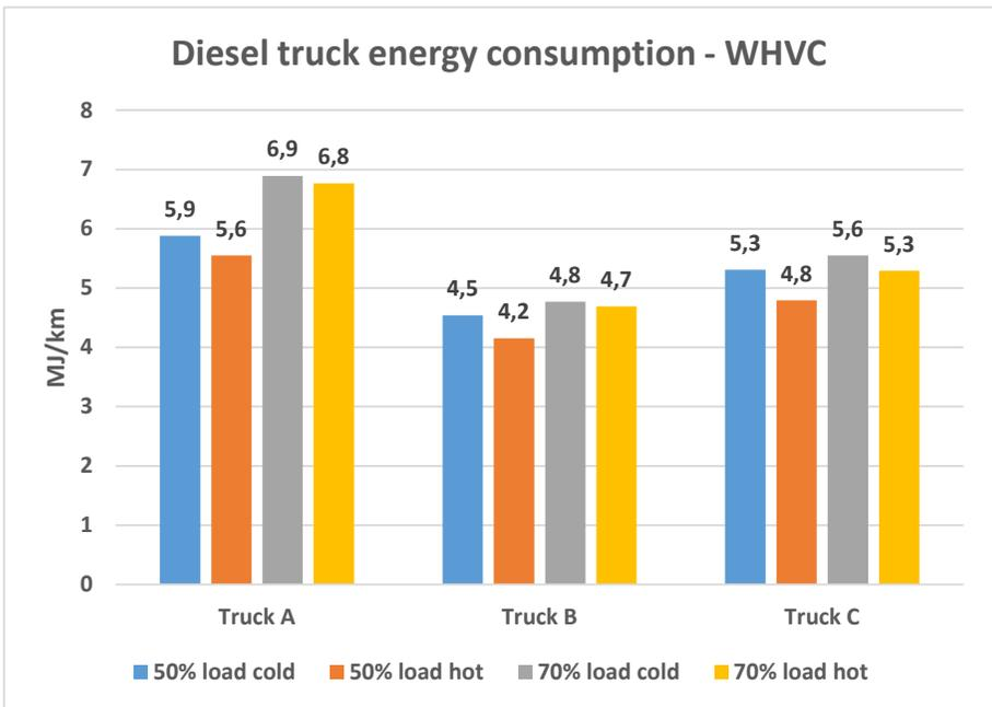
Figure 51: Diesel truck energy consumption, cold and hot WHVC.
