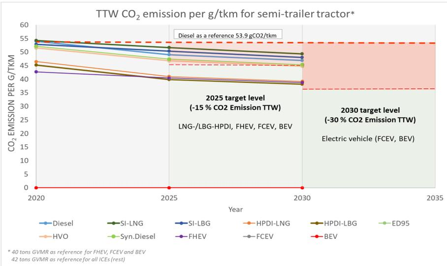
**Figure 131: CO<sub>2</sub> emissions in TTW basis per ton-kilometer for different powertrain and fuel options.**
