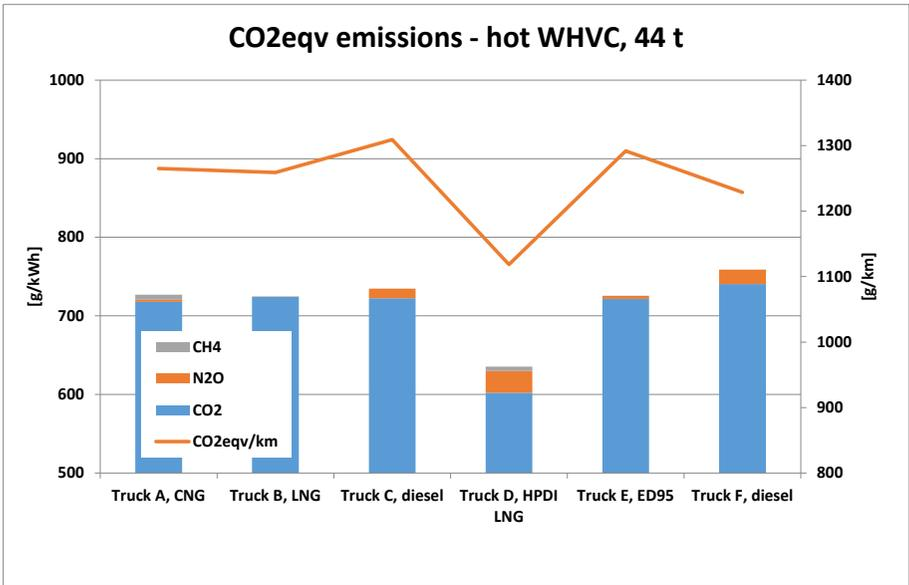
Figure 64: CO<sub>2</sub>eqv emissions (hot WHVC, 44 t). Values in g/kWh relate to work at the driving wheels.
