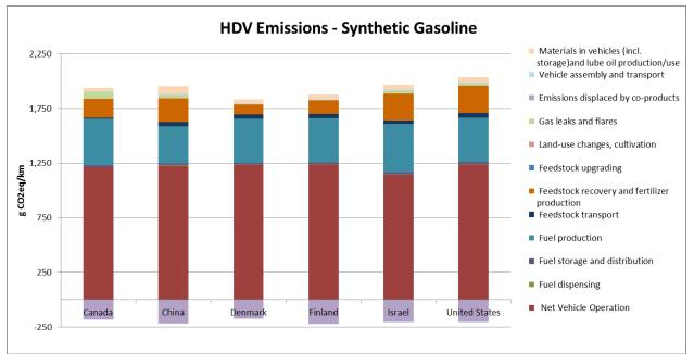
Figure 48: HDV Emissions for Synthetic Gasoline
