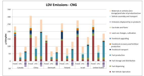
Figure 39: LDV Emissions for CNG
