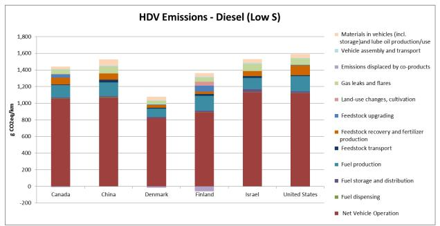
Figure 38: HDV Emissions for Low-S Diesel
