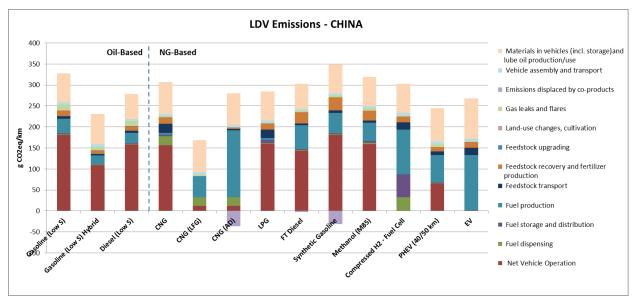
Figure 25: LDV Emissions for Natural Gas Pathways in China
