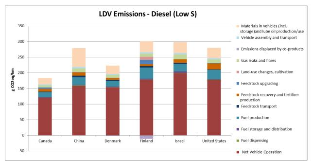
Figure 37: LDV Emissions for Low-S Diesel
