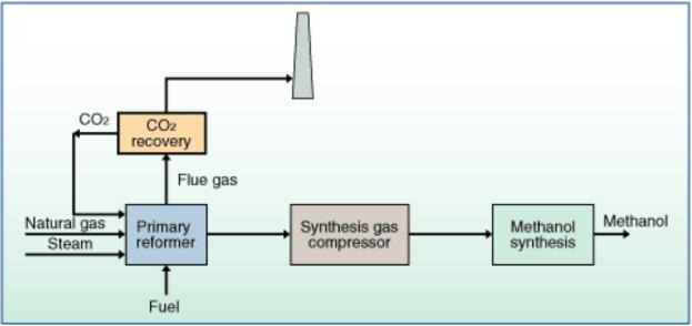
Figure 21: Methanol production from natural gas (Source: MHI Global)
