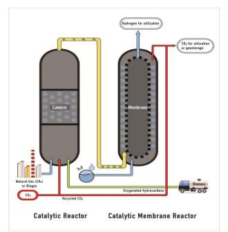
Figure 20: Hydrogen production from natural gas or biomass
