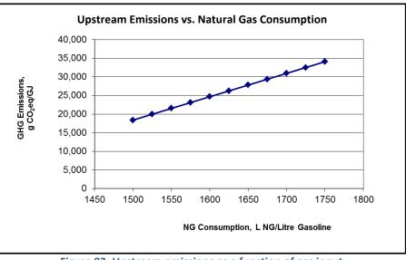
Figure 82: Upstream emissions as a function of gas input
