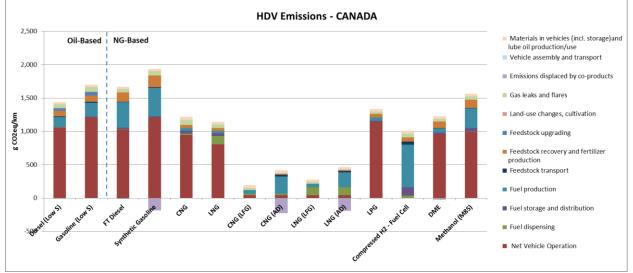
Figure 24: HDV Emissions for Natural Gas Pathways in Canada
