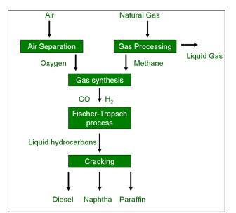
Figure 16: Diesel from natural gas using the Fischer-Tropsch method (Source: RBN Energy)
