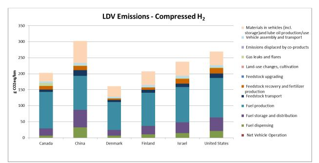
Figure 51: LDV Emissions for Compressed Hydrogen
