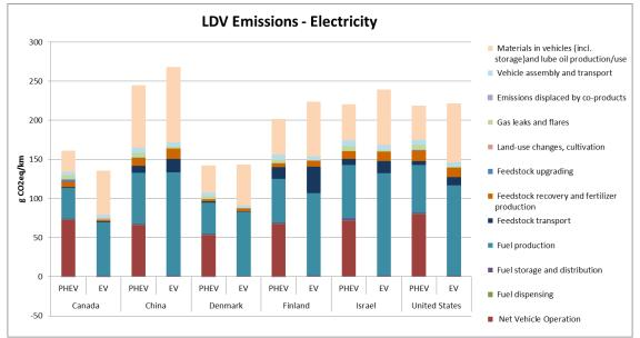
Figure 53: LDV Emissions for Electricity
