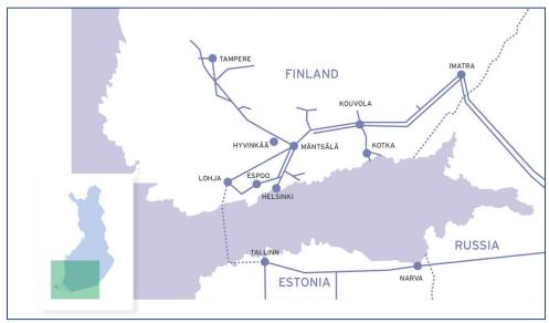
Figure 10: Finland's natural gas transmission network (Source: Gasum)
