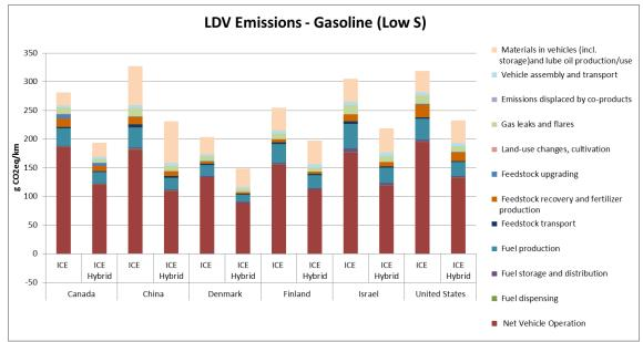
Figure 35: LDV Emissions for Low-S Gasoline
