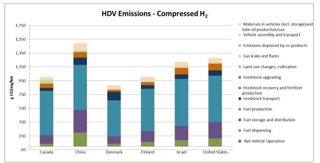
Figure 52: HDV Emissions for Compressed Hydrogen
