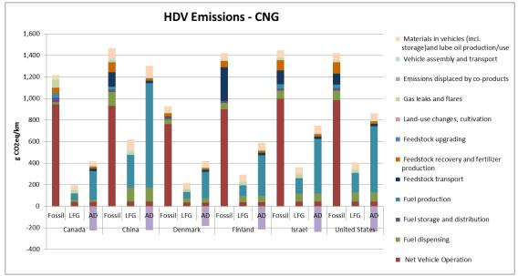
Figure 40: HDV Emissions for CNG
