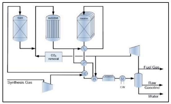
Figure 18: The Haldor Topsoe STG process (Source: Haldor Topsoe)
