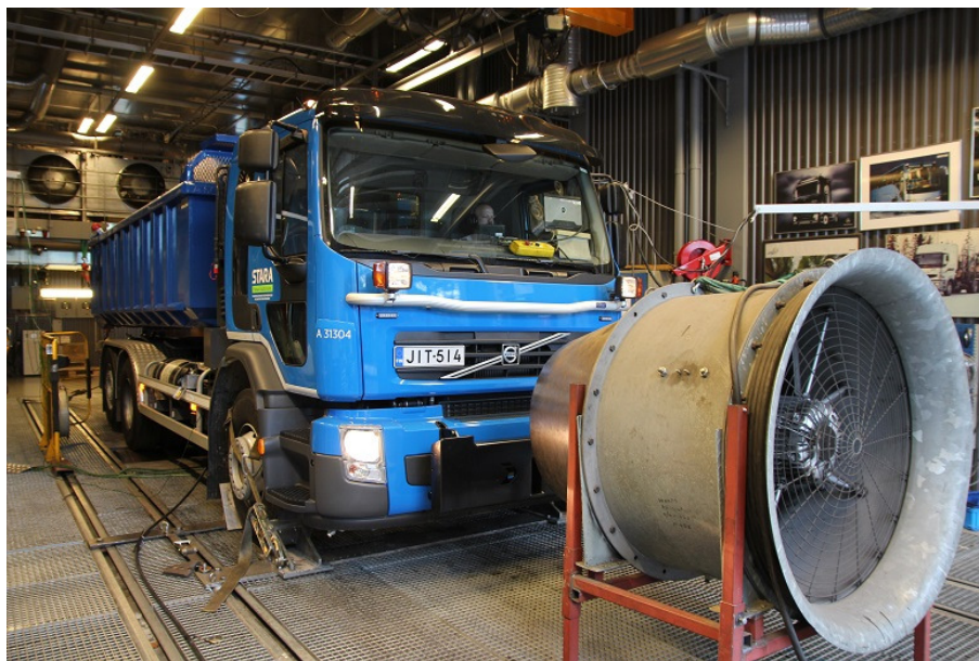
Figure 3: Volvo FE on VTT's heavy chassis dynamometer
