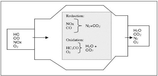
Figure 2. Chemical processes in a three way catalyst [1]
