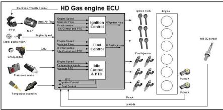
Figure 1. Example of the design for an ECU
