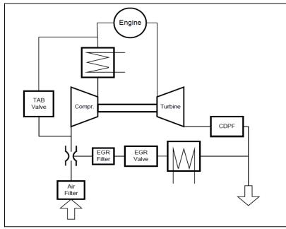
Figure 6. Basic lay-out of PACCOLD-EGR system
