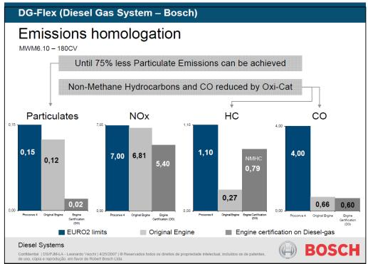
Figure 11. Emission results from Bosch Dual Fuel system eDG-Flex (Source: Bosch Brazil)
