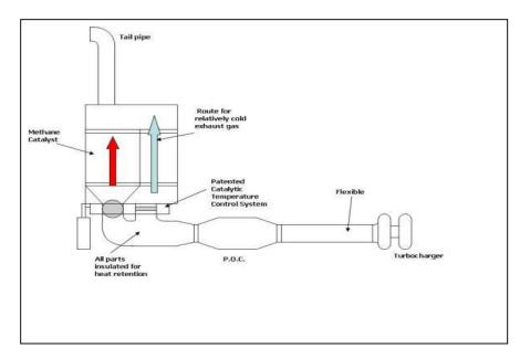
Figure 9. Hardstaff patented catalytic temperature control
