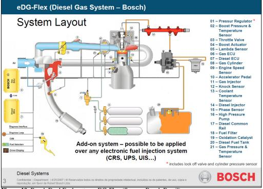
Figure 10. Bosch Dual Fuel system eDG-Flex (Source: Bosch Brazil)
