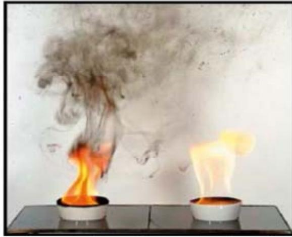
**Figure 10.19 - Burning of Conventional Diesel (left) and Paraffinic Diesel (right)**
