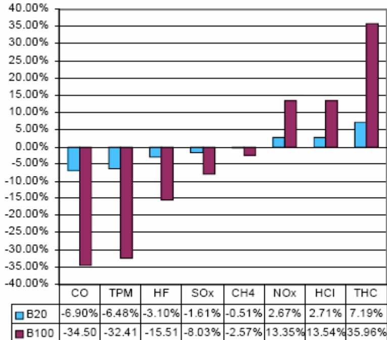
**Figure 6.3 - Life Cycle Air Emissions for Biodiesel Blends Compared to Petroleum Diesel (Sheehan et al 1998)**
