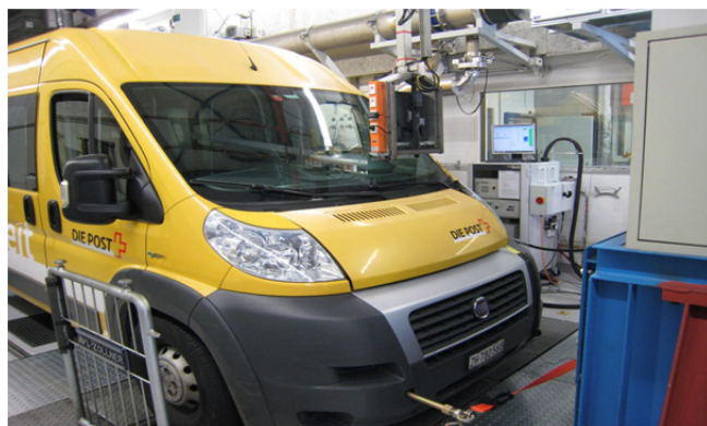
Fig. 5 Preparation of a Vehicle for a Field Test with CNG and Successive Switches to HCNG (2 vol% H 2 )
