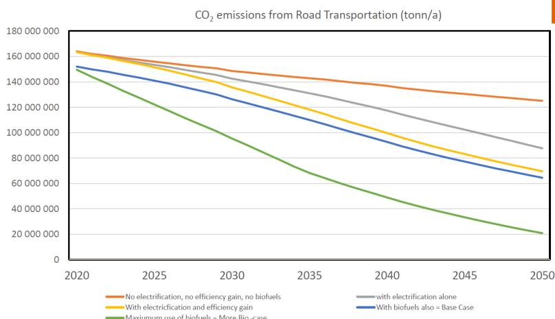
Fig. 2 Scenarios of CO<sub>2</sub> Emissions from Road Transportation for Germany
