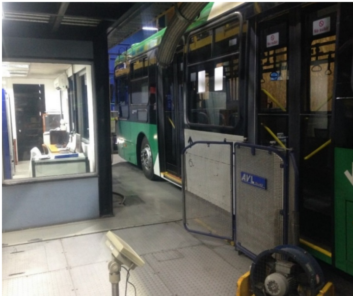
Fig. 1 Chilean Emission Laboratory for Heavy Vehicles with Chassis Dynamometer in the 3CV
