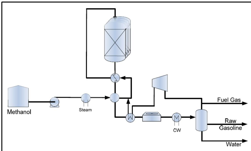
Figure 17: The Haldor Topsoe MTG process (Source: Haldor Topsoe)
