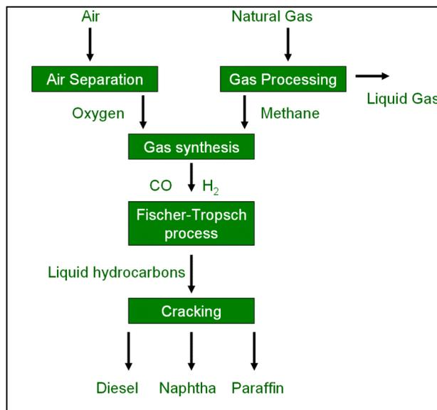
Figure 16: Diesel from natural gas using the Fischer-Tropsch method (Source: RBN Energy)
