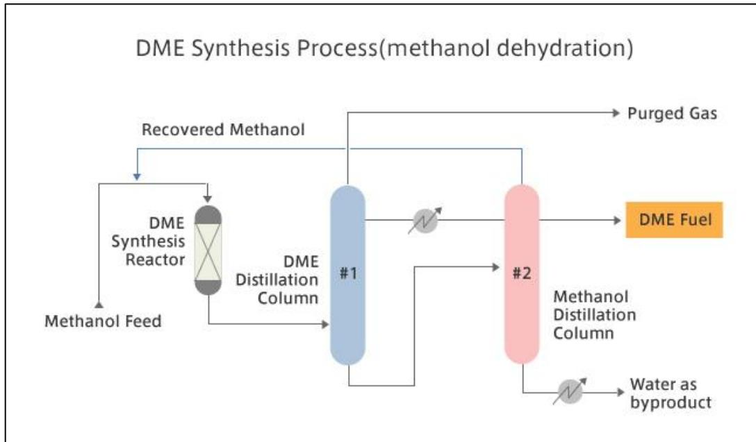
Figure 22: DME synthesis process via methanol dehydration (Source: JGC Corporation)
