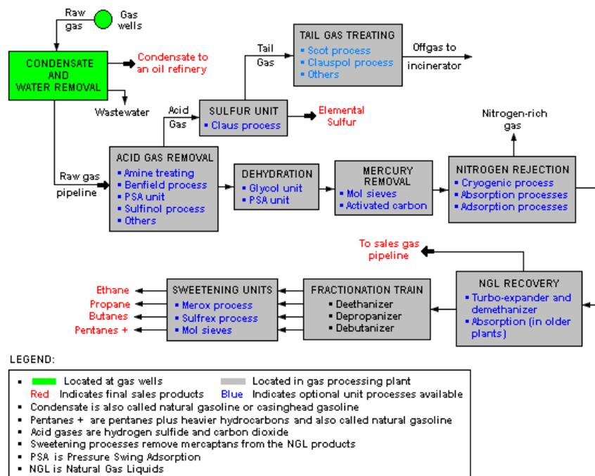
Figure 19: A schematic flow diagram of typical large natural gas processing plant (Source: Milton Beychok)
