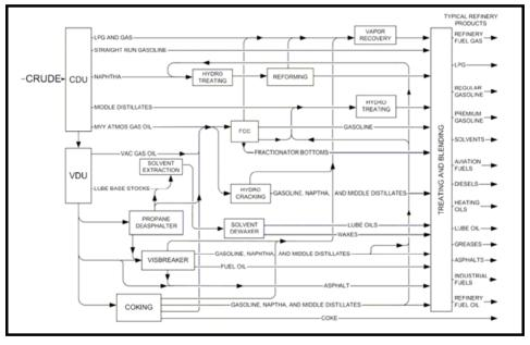
Figure 6-6 Typical Refinery Configuration
