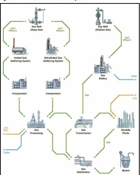
Figure 7-1 Natural Gas Production System
