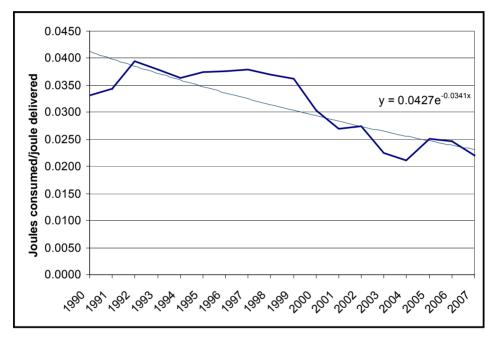
Figure 7-2 Pipeline Fuel Consumption
