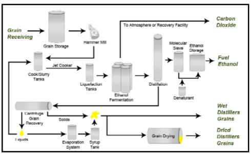
Figure 8-21 Ethanol Production Process
