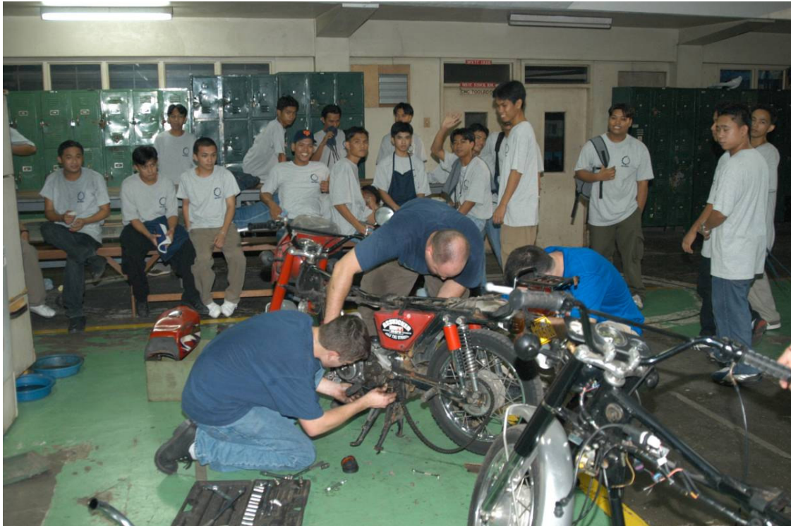
Figure 3 – Students at Don Bosco Technical College watch the CSU team install the prototype DI retrofit kit on an HD-III motorcycle
