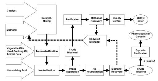
Figure 4.5 Biodiesel Production Process
