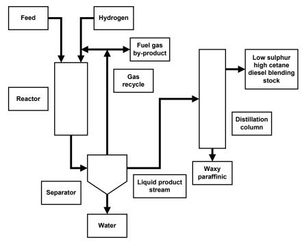
Several reactions occur in the process, including hydrocracking (breaking apart of large molecules), hydrotreating (removal of oxygen), and hydrogenation (saturation of double bonds). The catalyst used in the process is a conventional, commercial, refinery hydrotreating catalyst. Hydrogen is the only other input.
